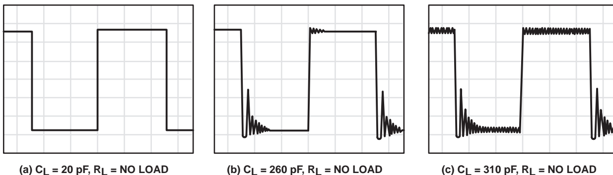
Figure 112. Effect of Capacitive Loads in Low-Bias Mode
