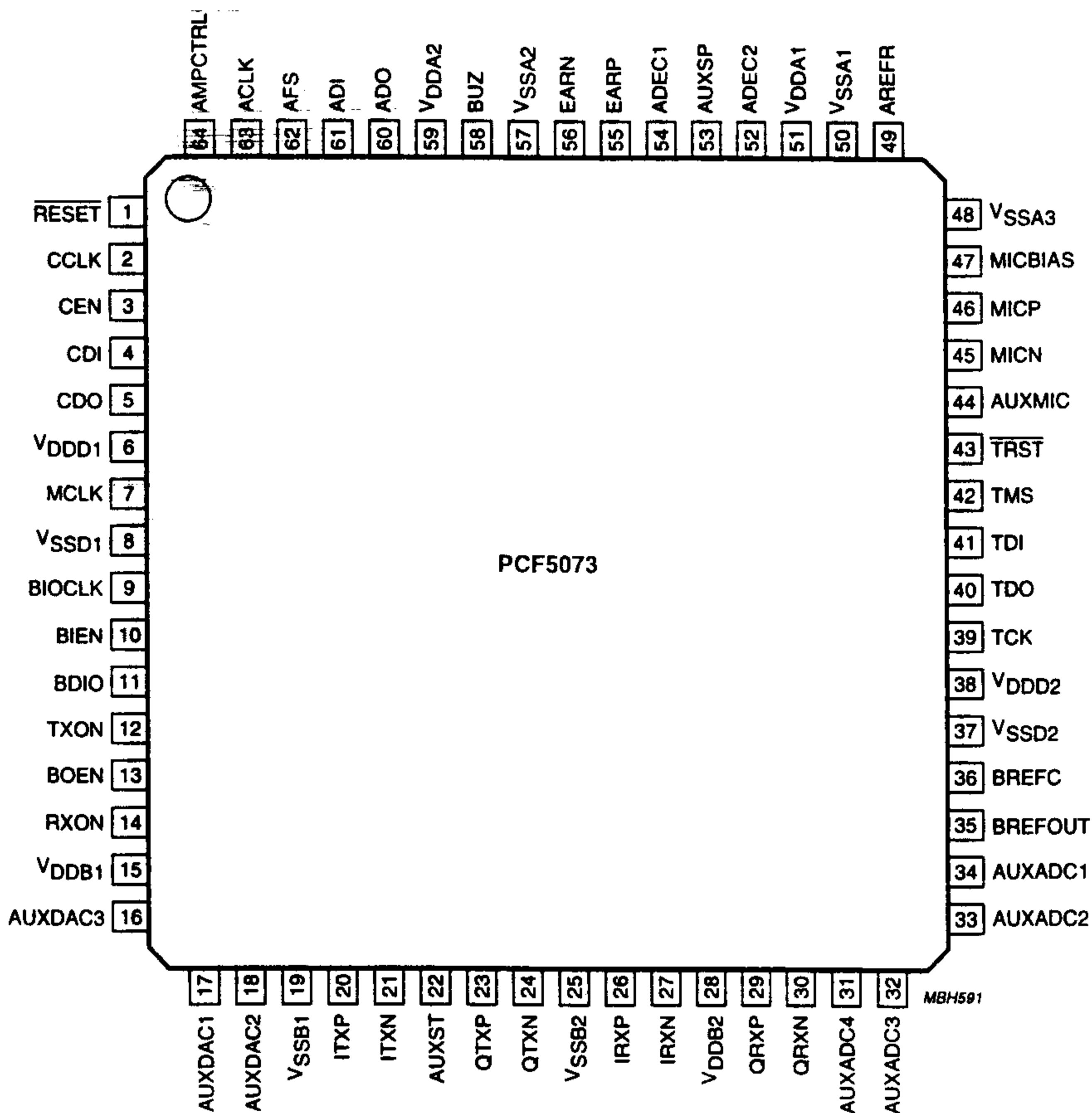
Fig.2 Pin configuration, LQFP64 package.
