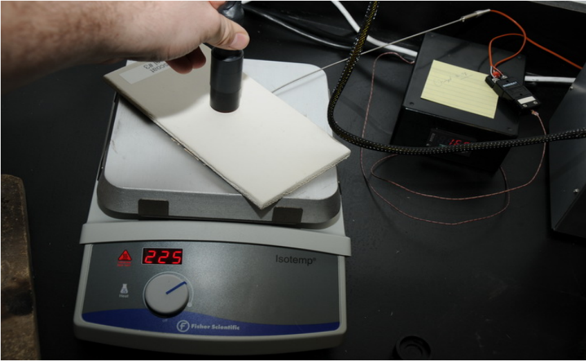
Figure 1. Test Set-up with TM probe on Center of Test Panel over a Hot Plate
