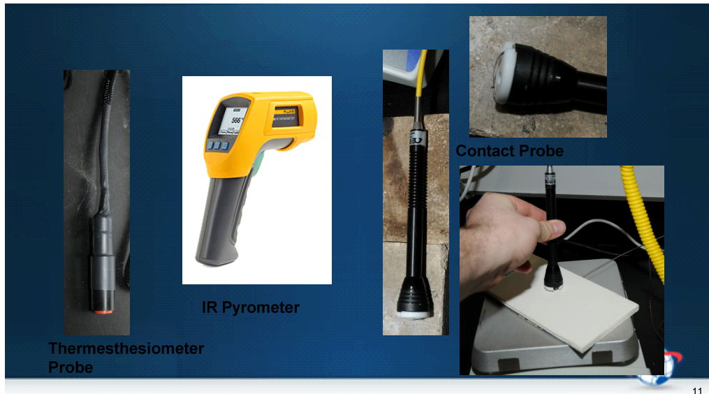
Figure 2. Photos of Temperature Probes and sensors
