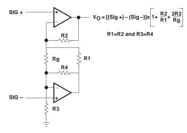
Figure 6. Two Op Amp Instrumentation Amplifier
