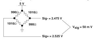
Figure 3. Sensor Output With No Load
