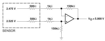
Figure 4. Thevenin Equivalent Shows Required Gain is 50% Higher
