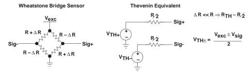
Figure 1. Wheatstone Bridge Sensor and Thevenin Equivalent
