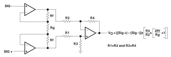
Figure 5. Three Op Amp Instrumentation Amplifier
