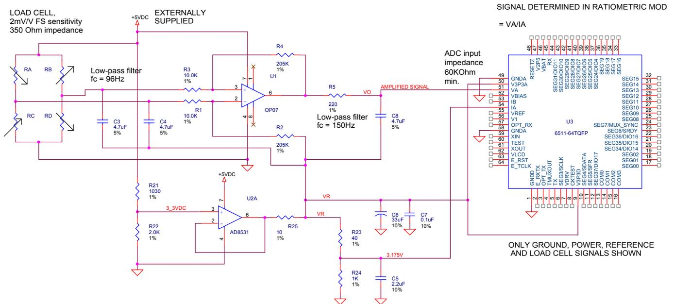
Figure 7: Ratiometric Measurement System
