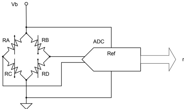
Figure 6: Ratiometric Measurement
