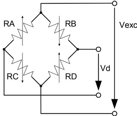
**Figure 2: Sensor Bridge Configuration**
