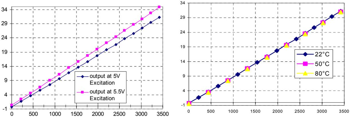
Figure 5: Sample Amplifier Output (left: Constant Temperature. Right: Variable Temperature)
