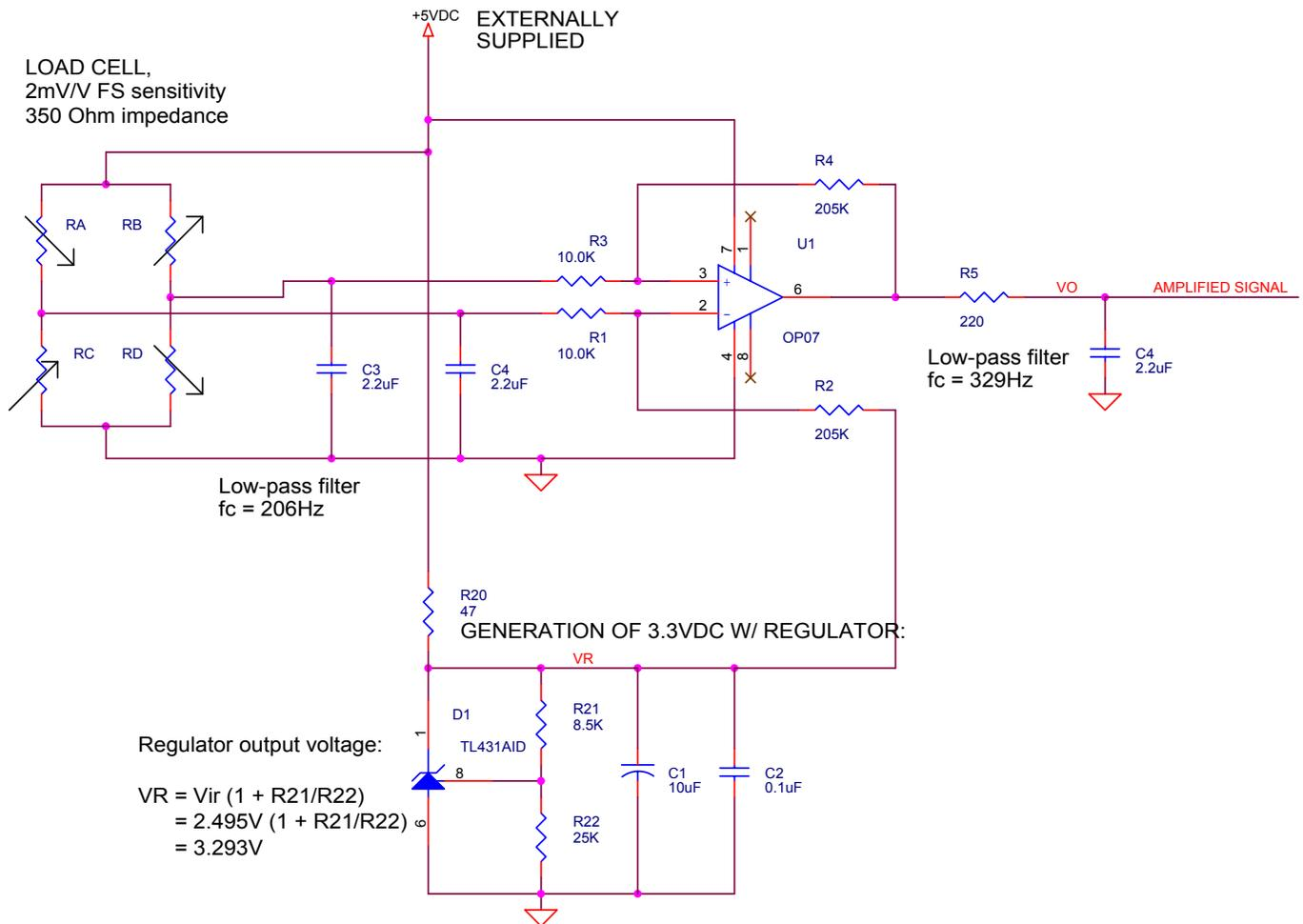
Figure 3: Simple Differential Amplifier and Reference Voltage Generator
