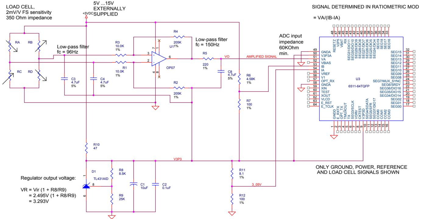
Figure 8: Ratiometric Measurement System
