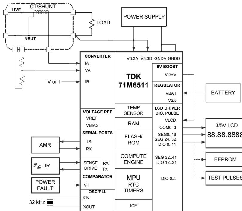
Figure 1: 71M6511 Used in an Energy Meter Application
