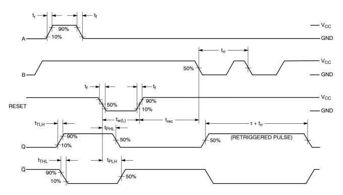
Figure 9. Switching Waveform
