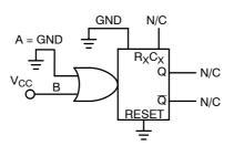
Figure 16. Connection of Unused Section
