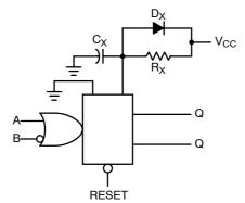
Figure 13. Discharge Protection During Power Down
