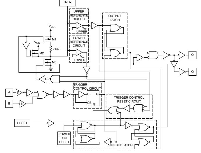
Figure 11. Logic Detail (1/2 the Device)
