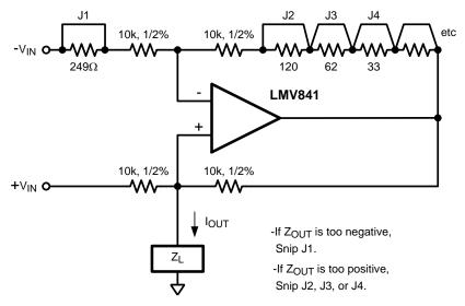
Figure 11. Trimming  $Z_{out}$  without a Trim-Pot
