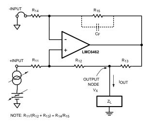
Figure 5. The "Improved Howland" Current Pump
