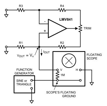
Figure 13. Good Test for Z<sub>OUT</sub> Using Floating Scope
