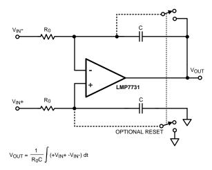
Figure 8. The Positive or Differential Integrator (not a Howland Circuit)
