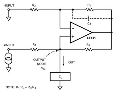
Figure 1. The Basic Howland Current Pump
