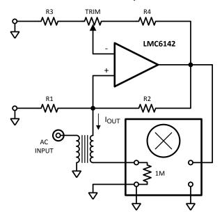
Figure 12. Transformer-Coupled Test for Z<sub>OUT</sub>
