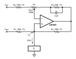
Figure 3. Basic Howland Current Pump with Trim of Z<sub>OUT</sub>
