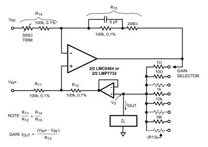
Figure 9. Multi-Range Current Pump
