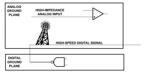
Figure 17–4. Broadcasting From PCB Traces
