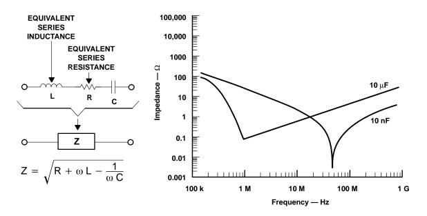
Figure 17–16. Capacitor Self Resonance
