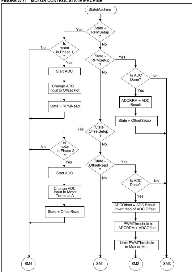
**MOTOR CONTROL STATE MACHINE** FIGURE A-7:
