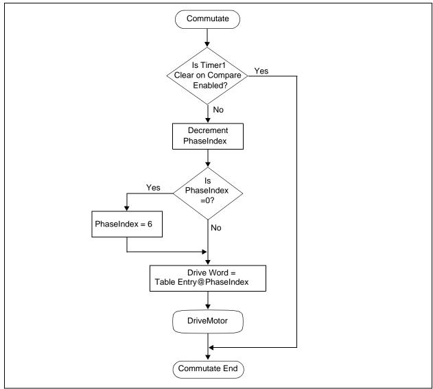
FIGURE A-3: MOTOR DRIVER CONTROL
