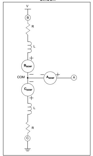
Figure 7 shows the equivalent circuit of the motor with coils B and C driven while coil A is undriven and available for BEMF measurement. At the commutation frequency the L's are negligible. The R's are assumed to be equal. The L and R components are not shown in the A branch since no significant current flows in this part of the circuit so those components can be ignored.
