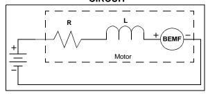
When the rotor is stationary, the only resistance to current flow is the impedance of the electromagnetic coils. The impedance is comprised of the parasitic resistance of the copper in the windings, and the parasitic inductance of the windings themselves. The resistance and inductance are very small by design, so start-up currents would be very large, if not limited.
