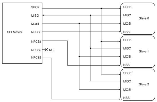
Figure 27-1. Block Diagram
