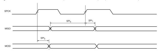
Figure 35-12. SPI Master Mode with (CPOL= NCPHA = 0) or (CPOL= NCPHA= 1)
