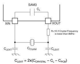
Where C<sub>PCB</sub> is the capacitance of the printed circuit board (PCB) track layout from the crystal to the SAM3 pin.
