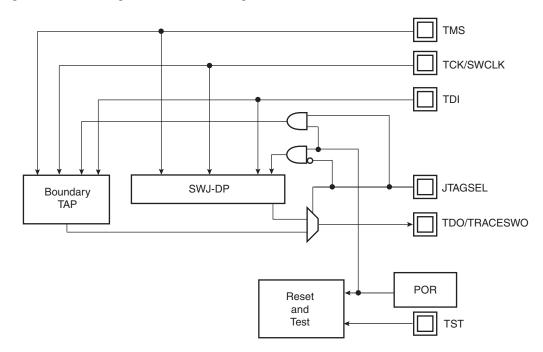
Figure 11-1. Debug and Test Block Diagram
