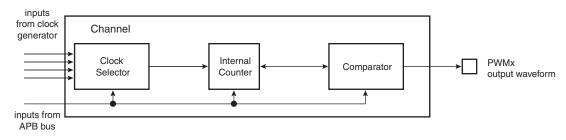
Figure 32-3. Functional View of the Channel Block Diagram
