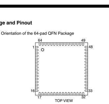
Orientation of the 64-pad QFN Package Figure 4-3.
