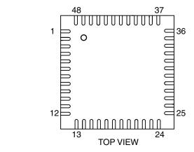
Figure 4-5. Orientation of the 48-pad QFN Package
