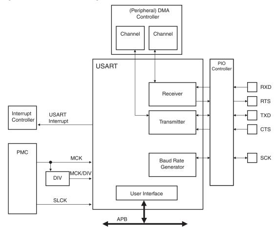
Figure 30-1. USART Block Diagram
