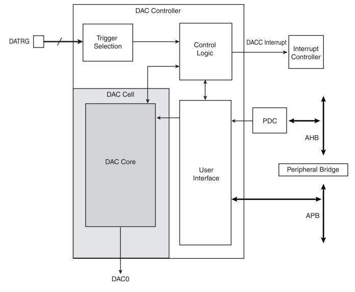
Figure 34-1. Digital-to-Analog Converter Controller Block Diagram
