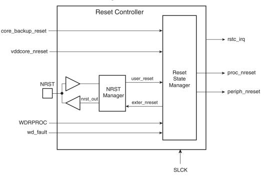
Figure 12-1. Reset Controller Block Diagram
