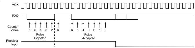
Figure 30-25. IrDA Demodulator Operations
