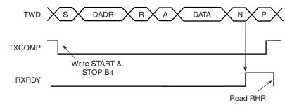
Figure 28-10. Master Read with Multiple Data Bytes
