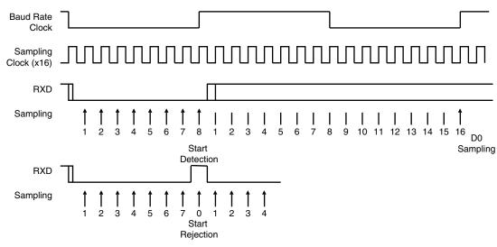
Figure 30-8. Asynchronous Start Detection
