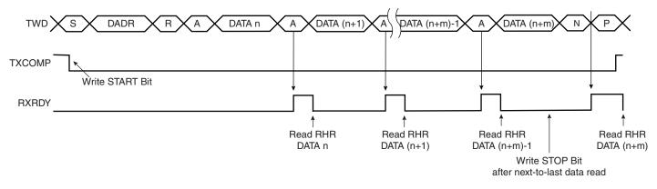
RXRDY is used as Receive Ready for the PDC receive channel.
