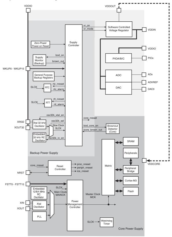
FSTT0 - FSTT15 are possible Fast Startup Sources, generated by WKUP0-WKUP15 Pins, but are not physical pins.
