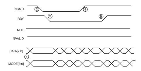
Figure 19-4. SAM3NxA (48 pins) Parallel Programming Timing, Write Sequence
