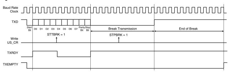
Figure 30-16. Break Transmission
