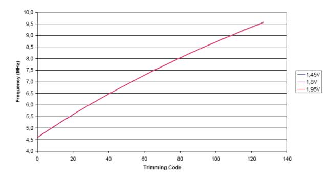
Figure 35-9. RC 8 MHz trimming
