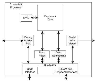
Figure 10-1. Typical Cortex-M3 Implementation
