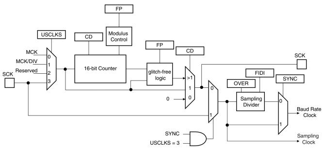
30.7.1.3 Baud Rate in Synchronous Mode or SPI Mode
