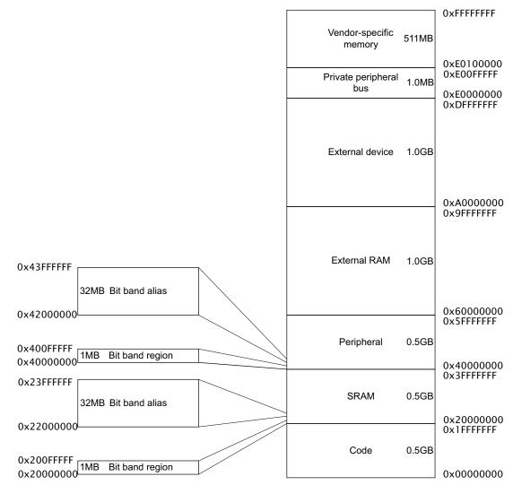
The regions for SRAM and peripherals include bit-band regions. Bit-banding provides atomic operations to bit data, see "Bit-banding" on page 59.
