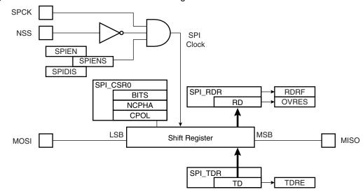
Figure 27-12. Slave Mode Functional Bloc Diagram
