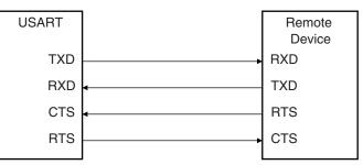
Figure 30-17. Connection with a Remote Device for Hardware Handshaking
