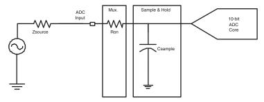
The user can drive ADC input with impedance of Zsource up to:
