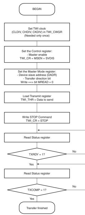
Figure 28-16. TWI Write Operation with Single Data Byte and Internal Address
