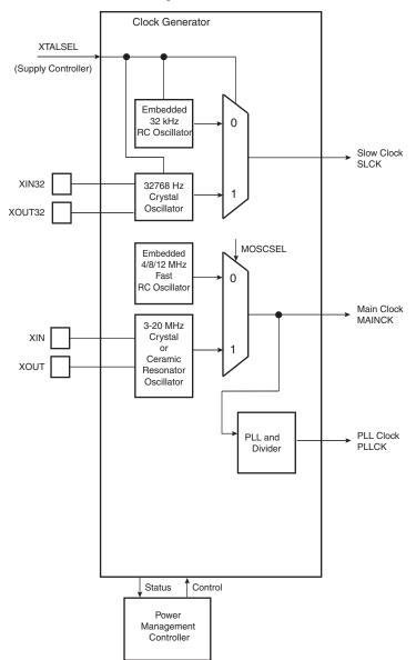
Figure 23-1. Clock Generator Block Diagram
