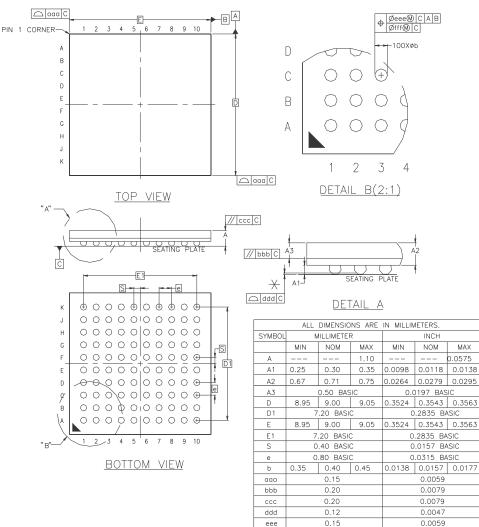
Figure 36-2. 100-ball TFBGA Package Drawing
