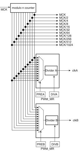
**Caution:** Before using the PWM macrocell, the programmer must first enable the PWM clock in the Power Management Controller (PMC).
