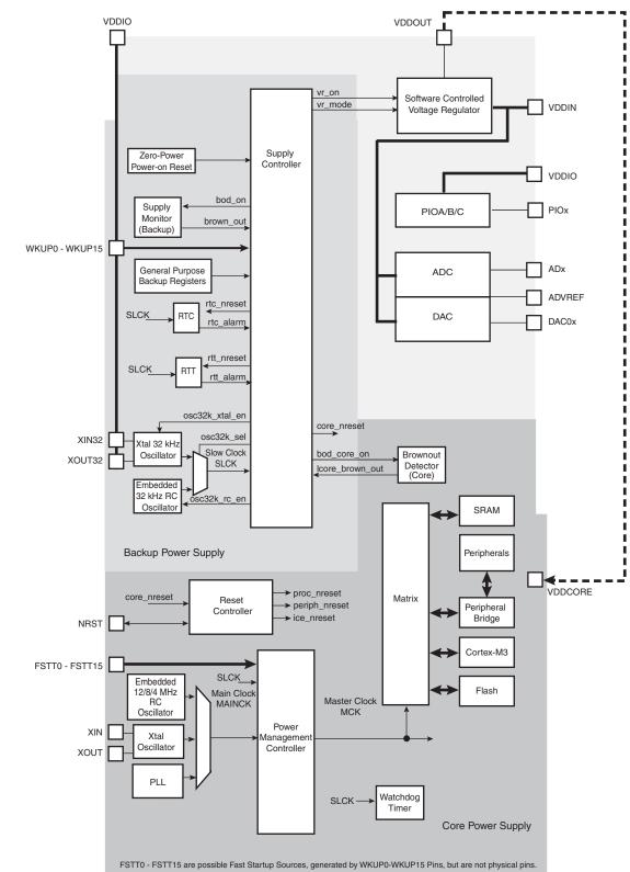
Figure 16-1. Supply Controller Block Diagram
