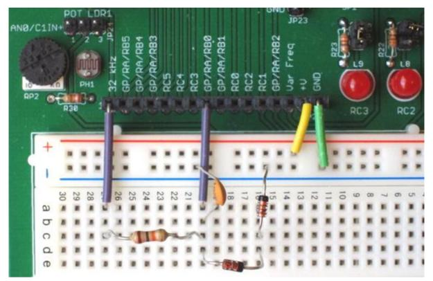
You should also remove the shunt from JP24 (disconnecting the pot or photocell from C1IN+), but leave JP19 in place (enabling the LED on RC3).
