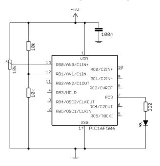
If you have the <u>Gooligum baseline training board</u>, you can implement this circuit by placing a shunt across pins 1 and 2 ('POT') of JP24, connecting the 10 k $\Omega$  pot (RP2) to C1IN+, and in JP19 to enable the LED on RC3.
