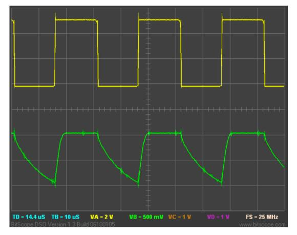
The top trace is the "clean" digital output of the clock circuit, and the degraded signal is below. It peaks at approximately 1 V.
