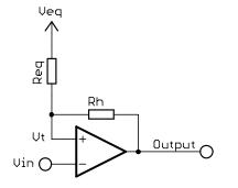
To calculate the high and low thresholds, recall Thévenin's theorem, which states that any two-terminal network of resistors and voltage sources can be replaced by a single voltage source, Veq, in series with a single resistor, Req.
