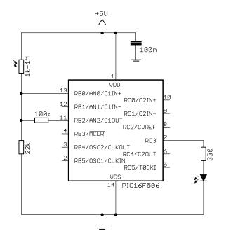
The effect is similar to that for threshold voltage feedback. At that level of illumination, the potential divider formed by the LDR and the 22 k $\Omega$  resistor is equivalent to a source (input) voltage of 0.6 V, connected to C1IN+ via a resistance of:
