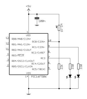
To test whether the input is within limits, we will first configure the programmable voltage reference to generate the "low" threshold voltage, compare the input with this low level, and then reconfigure the voltage reference to generate the "high" threshold and compare the input with this higher level.
