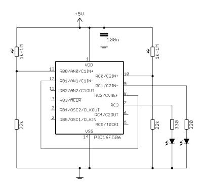
But although no internal connection is available, that doesn't rule out an external connection – and as we saw above, the programmable reference can be made available on the CVREF pin.
