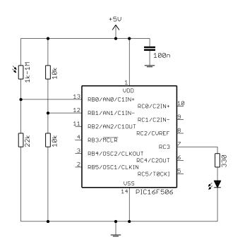
photocell (PH1) and 22 k $\Omega$  resistor in the lower left of the board to C1IN+.
