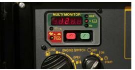
The control panel on this Subaru Robin unit provides information about its output and the hours it has run as well as the engine controls.
