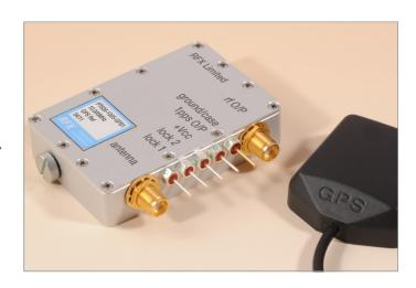
The PT626 - GPS sets a new benchmark for miniature frequency standards. The combination of regulation through the aquisition of GPS data, the storage of control levels, miniature size and integrated OCXO provides a component level module for incorporation into OEM equipment.
