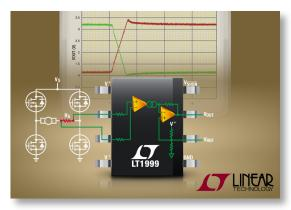
The LT1999 accurately measures fast switching currents in H-bridge motor controls, switching power supplies, solenoids and battery chargers. It features a –5V to 80V input common mode voltage range, 2MHz bandwidth, less than 1.5mV offset voltage and 0.5% gain error over temperature. With more than 80dB common mode rejection at 100kHz, the LT1999 maintains outstanding accuracy even in the presence of large square wave input voltages.
