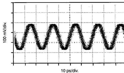
Fig. 2 Output 50 GHz signal of dynamic divider at 100 GHz input
