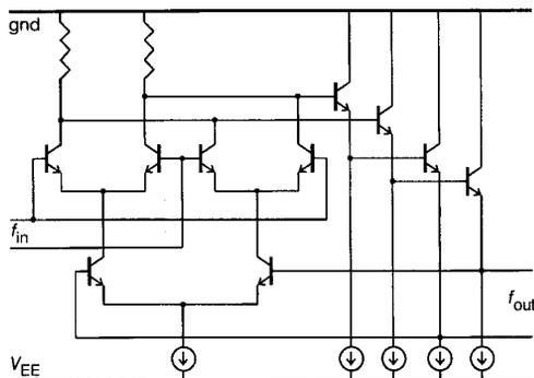
Fig. 1 Dynamic divider circuit diagram
