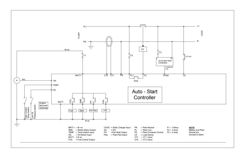
Figure 3 Typical Auto-Start Installation
