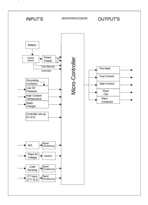
Figure 2 Block Diagram Auto-Start
