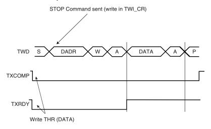
Figure 28-7. Master Write with Multiple Data Bytes
