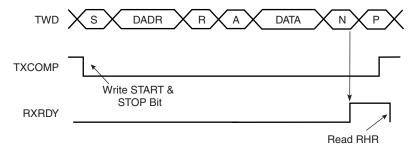
Figure 28-10. Master Read with Multiple Data Bytes
