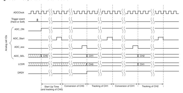
Figure 33-2. Sequence of ADC conversions
