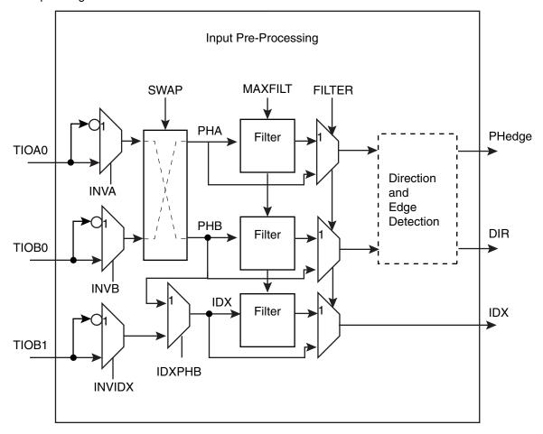
Input filtering can efficiently remove spurious pulses that might be generated by the presence of particulate contamination on the optical or magnetic disk of the rotary sensor.
