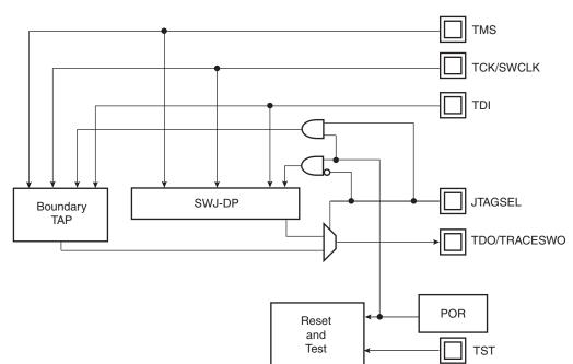
Figure 11-1. Debug and Test Block Diagram
