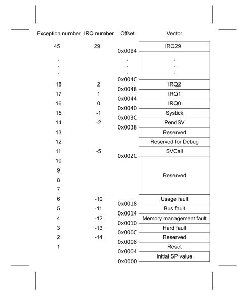
On system reset, the vector table is fixed at address 0x00000000. Privileged software can write to the VTOR to relocate the vector table start address to a different memory location, in the range 0x00000080 to 0x3FFFFF80, see "Vector Table Offset Register" on page 170.
