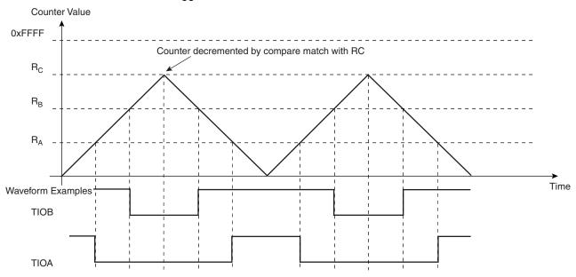
Figure 31-14. WAVSEL = 11 With Trigger
