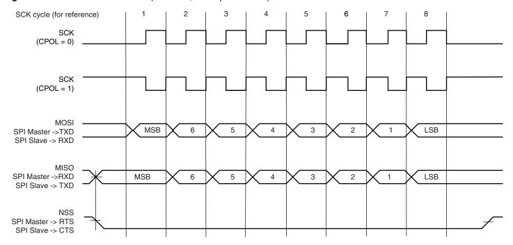
Figure 30-29. SPI Transfer Format (CPHA=0, 8 bits per transfer)
