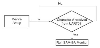
The SAM-BA Boot program uses the internal 12 MHz RC oscillator as source clock for PLL. The MCK runs from PLL divided by 2. The core runs at 48 MHz.
