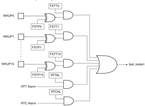
Figure 24-3. Fast Startup Circuitry
