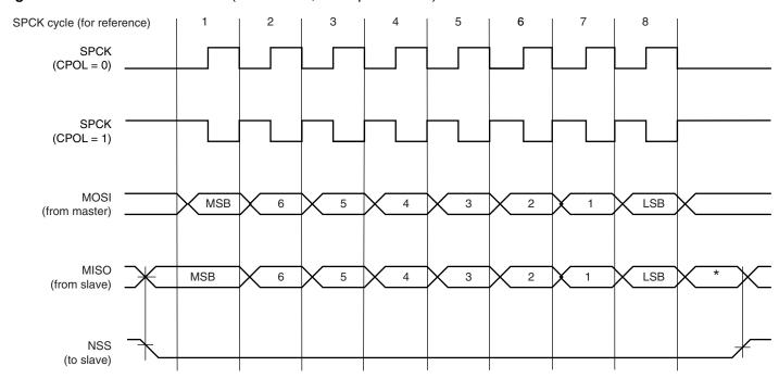
**Figure 27-3.** SPI Transfer Format (NCPHA = 1, 8 bits per transfer)
