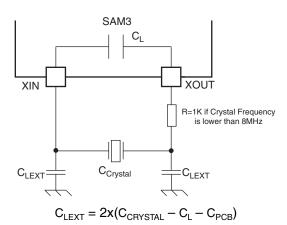
Where  $C_{PCB}$  is the capacitance of the printed circuit board (PCB) track layout from the crystal to the SAM3 pin.
