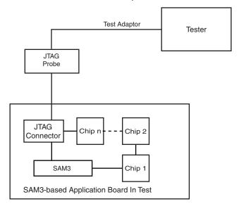
Figure 11-3. Application Test Environment Example
