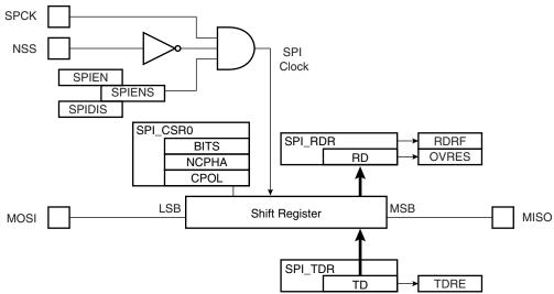
Figure 27-12. Slave Mode Functional Bloc Diagram
