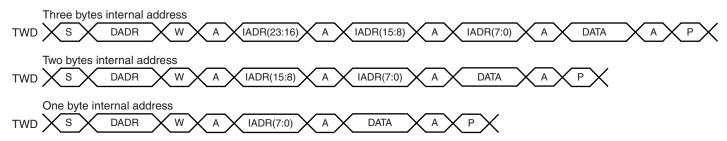
Figure 28-12. Master Read with One, Two or Three Bytes Internal Address and One Data Byte
