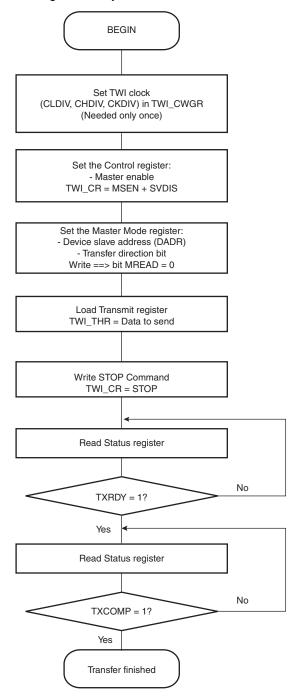
Figure 28-16. TWI Write Operation with Single Data Byte and Internal Address
