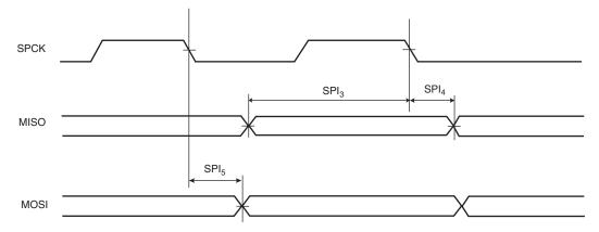
Figure 35-14. SPI Slave Mode with (CPOL=0 and NCPHA=1) or (CPOL=1 and NCPHA=0)
