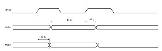
Figure 35-13. SPI Master Mode with (CPOL = 0 and NCPHA=1) or (CPOL=1 and NCPHA= 0)
