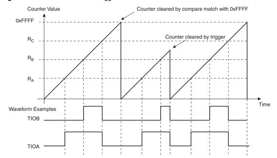
Figure 31-8. WAVSEL= 00 with trigger
