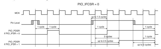
Figure 26-6. Input Debouncing Filter Timing
