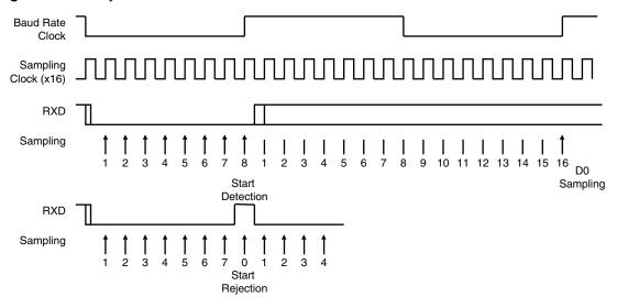
Figure 30-9. Asynchronous Character Reception
