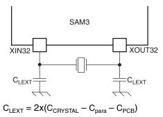
Where  $C_{PCB}$  is the capacitance of the printed circuit board (PCB) track layout from the crystal to the SAM3 pin.
