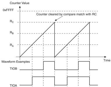
**Figure 31-9.** WAVSEL = 10 Without Trigger
