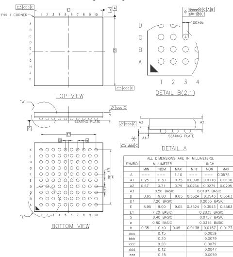
Figure 36-2. 100-ball TFBGA Package Drawing
