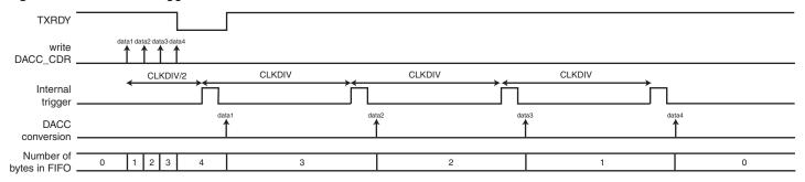
Figure 34-3. External trigger
