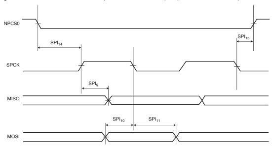
Figure 35-15. SPI Slave Mode with (CPOL = NCPHA = 0) or (CPOL = NCPHA = 1)
