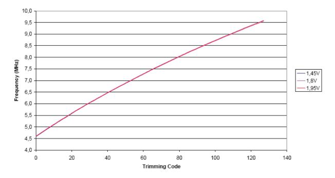
Figure 35-10. RC 12 MHz trimming
