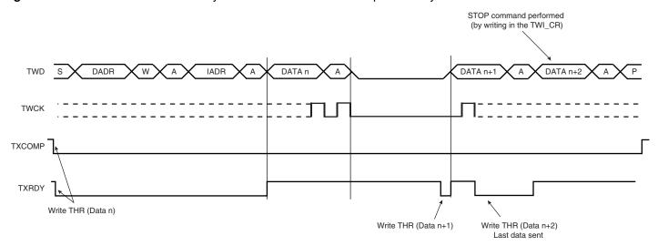
TXRDY is used as Transmit Ready for the PDC transmit channel.
