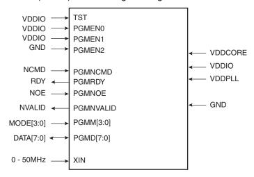
Figure 19-2. SAM3NxB/C (64/100 pins) Parallel Programming Interface
