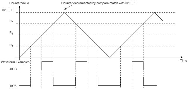
Figure 31-12. WAVSEL = 01 With Trigger
