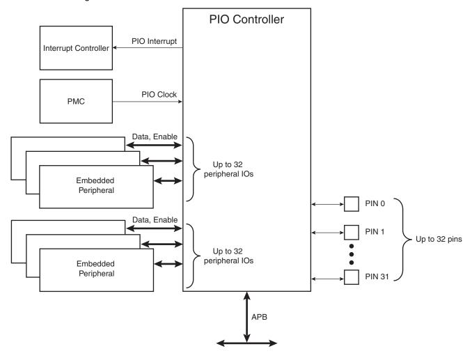
Figure 26-2. Application Block Diagram
