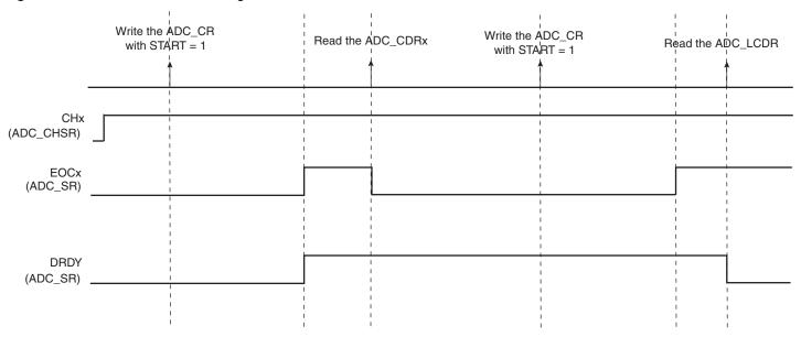
If the ADC\_CDR is not read before further incoming data is converted, the corresponding Overrun Error (OVREx) flag is set in the Overrun Status Register (ADC\_OVER).
