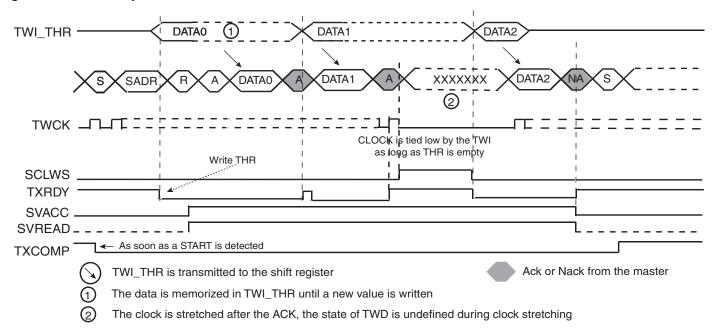
Notes: 1. TXRDY is reset when data has been written in the TWI\_THR to the shift register and set when this data has been acknowledged or non acknowledged.
