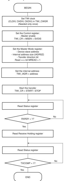
Figure 28-20. TWI Read Operation with Multiple Data Bytes with or without Internal Address
