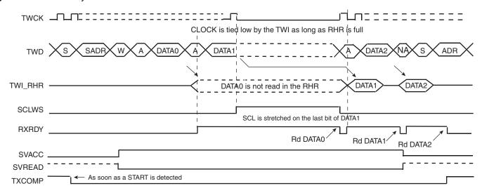
Notes: 1. At the end of the read sequence, TXCOMP is set after a STOP or after a REPEATED\_START + an address different from SADR.
