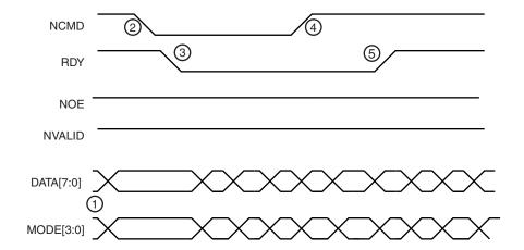
Figure 19-4. SAM3NxA (48 pins) Parallel Programming Timing, Write Sequence
