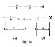
Thus the self-inductance of such a circuit is independent of the width of the tapes. If the tapes are separated by the distance b, Fig. 48 (3), equal to the width of the tapes,  $R_2 = 1.95653b$  and L = 8.685l.
