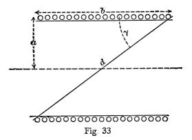
single layer solenoid. It is, like the others, a current sheet formula, and requires correction by (80) for a winding of wire, but applies to a solenoid of any length. Changing the notation slightly Lorenz's formula as originally given is as follows:
