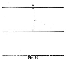
length and mean radius. The first is a single winding of thin tape and the self-inductance, calculated by a current sheet formula, is  $L_s$ . The second is a single layer of wire of square section (length b, depth c, and b/c turns) and its self-inductance is  $L_u$ , the current being supposed uniformly distributed over the area of the square conductors. The third is a winding
