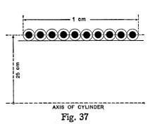
The difference of less than one in a million between the results obtained by formulas (69) and (80) combined and formula (81) is a good check on the corrections of (80), which amount in this case to more than I per cent of the value of the self-inductance. Formula (69) for as short a coil as this is very accurate, the next term, the fourth term of (71), being inappreciable.
