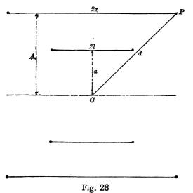
solenoid. S depends upon x/A, a/A, and A/d; that is, upon the relative sizes of the inner circle and the solenoid and the shape of the solenoid. If we have the value of RS, or K of equation (57) for a given solenoid and circle, we can get M by multiplying by  $a^2n_1$ , and for any other system of similar shape but different size by multiplying the same value of K by  $a^2n_1$ . The values of the constant K for various values of a/A and x/A are given in Table III, page 193.
