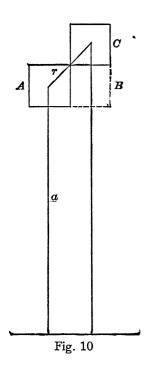
The mutual inductance of two coaxial coils adjacent or very near can sometimes be obtained by means of the geometric mean distances. This method is accurate only when the sections are very small relatively to the radius. It can often be used to advantage in testing other formulas, but not often in determining the mutual inductance of actual coils.
