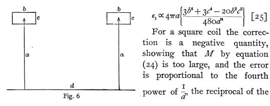
distance between the mean planes of the coils. For a rectangular coil in which b is greater than c the correction is negative so long as b is not more than 2.5 times c. When b is still larger with respect to c the correction becomes plus, the value of M by (24) being too small.
