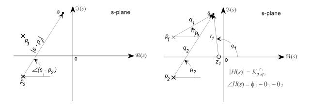
Figure 5: (a) Definition of s-plane geometric relationships in polar form, (b) Geometric evaluation of the transfer function from the pole-zero plot.
