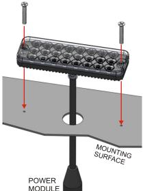
Drill a 0.625" diameter hole in the mounting surface to pass the cable through.
