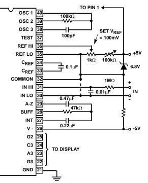
Since low TC zeners have breakdown voltages ~ 6.8V, diode must be placed across the total supply (10V). As in the case of Figure 12, IN LO may be tied to either COMMON or GND.
