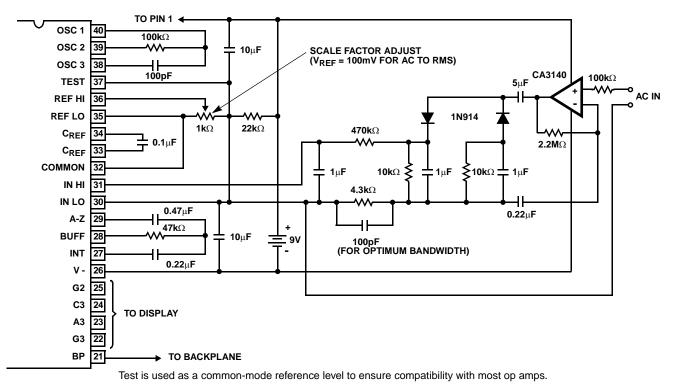
FIGURE 21. AC TO DC CONVERTER WITH ICL7106
