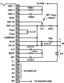
Values shown are for 200mV full scale, 3 readings/sec., floating supply voltage (9V battery).
