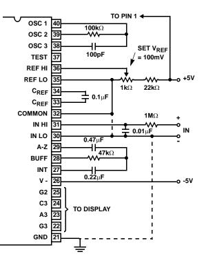
Values shown are for 200mV full scale, 3 readings/sec. IN LO may be tied to either COMMON for inputs floating with respect to supplies, or GND for single ended inputs. (See discussion under Analog COMMON).
