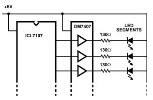
FIGURE 22. DISPLAY BUFFERING FOR INCREASED DRIVE CURRENT
