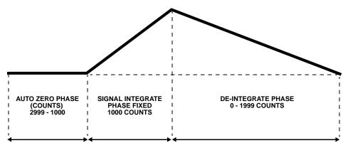
TOTAL CONVERSION TIME = 4000 x t<sub>CLOCK</sub> = 16,000 x t<sub>OSC</sub>
