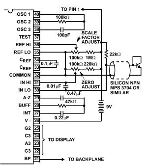
A silicon diode-connected transistor has a temperature coefficient of about  $-2mV/^{o}C$ . Calibration is achieved by placing the sensing transistor in ice water and adjusting the zeroing potentiometer for a 000.0 reading. The sensor should then be placed in boiling water and the scale-factor potentiometer adjusted for a 100.0 reading.
