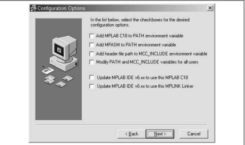
A detailed description of the available configuration options is shown in Table 2-2. Select the components to be installed, then click **Next**.
