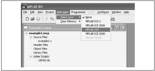
FIGURE 3-19: SELECT DEBUGGER, MPLAB SIM OPTION
