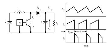
Figure 6. Boost Regulator and Associated I/V Waveforms
