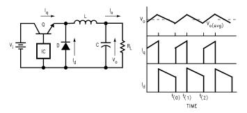
Figure 5. Buck Regulator Circuit with Voltage and Current Waveforms
