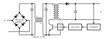
Figure 9. Complete Isolated Flyback Switching Supply
