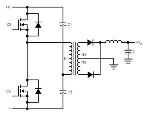
Figure 13. Half-Bridge Converter Circuit
