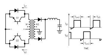
Figure 12. Push-Pull Converter
