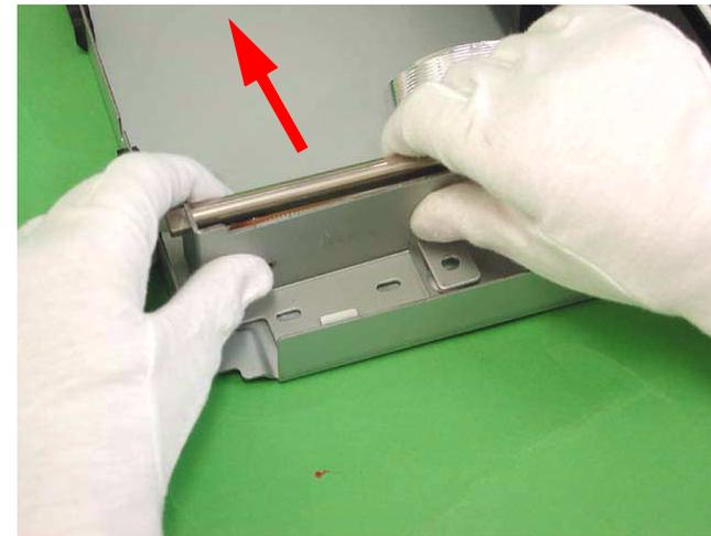
Figure 4-21. Driven Pulley Assembly Removal (2)
