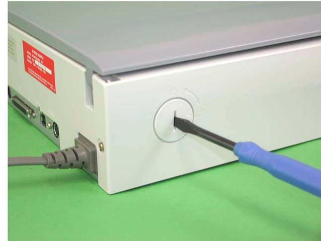
Figure 4-2. Carriage Lock Position
