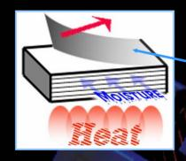
Potential delamination of stack with heat and moisture. More a potential problem in large sizes.
