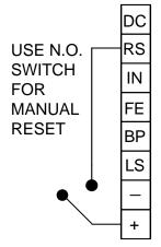
We have talked about "resetting" the DPA several times earlier in this manual. Reset recovers from two latching alarm conditions: the standard fourth stage condition at the end of time range two and the special forbidden condition alarm signal (see Section 4.1). The board will receive a reset signal when +V is input to terminal RS.
