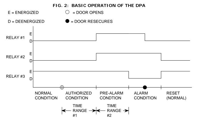
A single graph cannot show all the operating features of the DPA, but Figure 2 does display the basics of the product. Note the events that distinguish between the conditions. The authorized condition begins when the door opens or becomes insecure. Time range one defines the length of the authorized condition unless the door recloses before the end of time range one, in which
