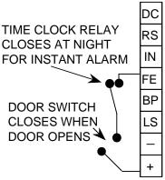
reads the forbidden condition and goes into instant alarm. Recovery is by reclosing the door and sending a reset input to the DPA. We prefer the use of the duress input as using the forbidden condition technique reduces the security of the door. If, for example, the lock failed to engage, this would not be reported as the time clock shunts this signal at night.
