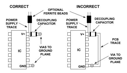
**Figure 12.66:** Localized High Frequency Supply Filter(s) Provides Optimum Filtering and Decoupling via Short Low-Inductance Path (Ground Plane)
