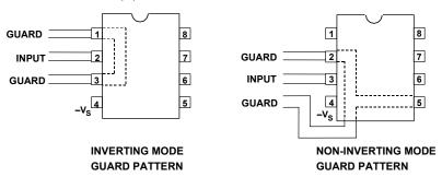
Figure 12.16: PCB Guard Patterns for Inverting and Noninverting Mode Op Amps Using Eight Pin SOIC (R) Package
