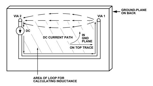
Figure 12.61: DC Current Flow for Figure 12.60
