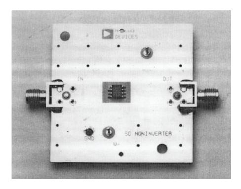
Fig. 12.30a: AD8001AR (SOIC) Evaluation Board—Top View
