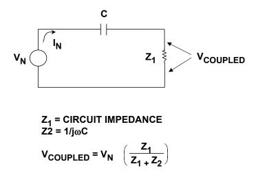
Figure 12.25: Capacitive Coupling Equivalent Circuit Model
