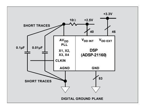
Figure 12.59: Grounding DSPs with Internal Phase-Locked-Loops (PLLs)
