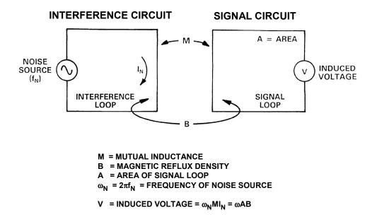
Figure 12.20: Basic Principles of Inductive Coupling
