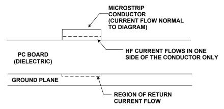
Figure 12.32: Skin Depth in a PCB Conductor
