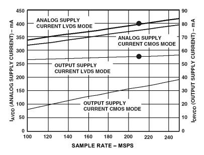
TOTAL CURRENT @ 210MSPS, LVDS MODE = 55mA + 400mA = 455mATOTAL POWER DISSIPATION =  $3.3V \times 455mA = 1.5W$
