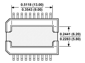
Figure 12.75: Bottom View of AD8016 20-Lead PSOP3 Package Showing Copper Slug for Aid in Heat Transfer (Central Grayed Area)
