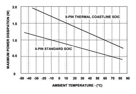
Figure 12.73: Thermal Rating Curves for Standard (Lower) and ADI Thermal Coastline (Upper) 8-Pin SOIC Packages
