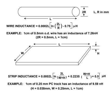
Figure 12.18: Wire and Strip Inductance Calculations
