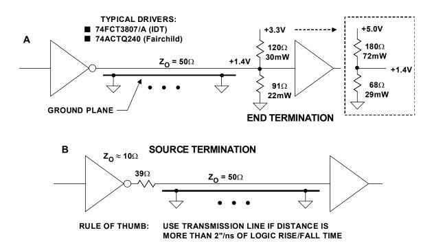
50  $\Omega$  PC BOARD TRANSMISSION LINE DELAY  $\approx$  1ns / 7"
