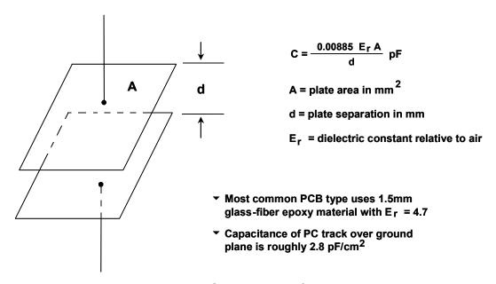
Figure 12.24: Capacitance of two parallel plates
