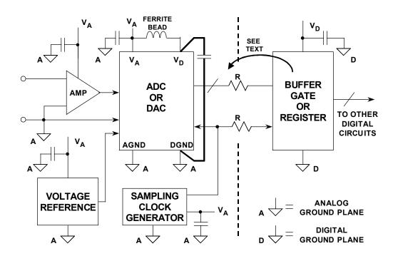
Figure 12.54: Grounding and Decoupling Points
