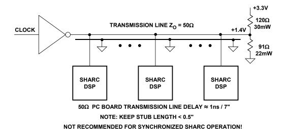
Figure 12.43: Clock Distribution Using End-of-Line Termination
