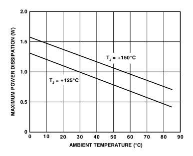
Figure 12.72: Thermal Rating Curves for AD8017AR Op Amp
