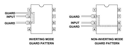
Figure 12.15: PCB Guard Patterns for Inverting and Noninverting Mode Op
