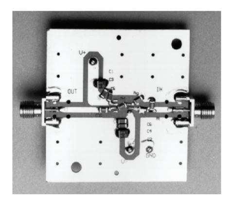
Fig. 12.30b: AD8001AR (SOIC) Evaluation Board—Bottom View
