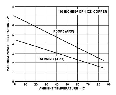
Figure 12.74: Thermal Characteristic Curves for the AD8016 BATWING (Lower) and PSOP3 (Upper) Packages, for T<sub>J(Max)</sub> Equal to 125 ℃
