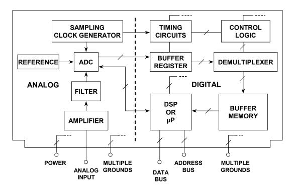
Figure 12.1: Analog and Digital Circuits Should Be Partitioned on PCB Layout
