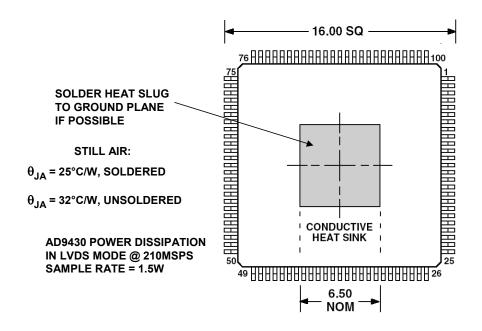
Figure 12.81: AD9430 100-Lead e-PAD TQFP
