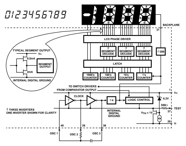
FIGURE 7. ICL7106 DIGITAL SECTION
