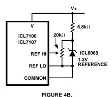
FIGURE 4. USING AN EXTERNAL REFERENCE
