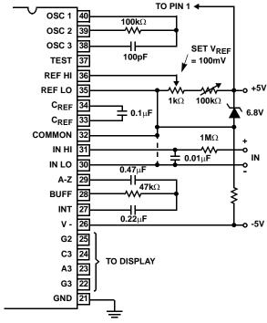
Since low TC zeners have breakdown voltages  $\sim$  6.8V, diode must be placed across the total supply (10V). As in the case of Figure 12, IN LO may be tied to either COMMON or GND.
