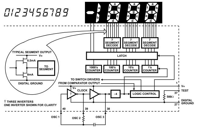
FIGURE 8. ICL7107 DIGITAL SECTION
