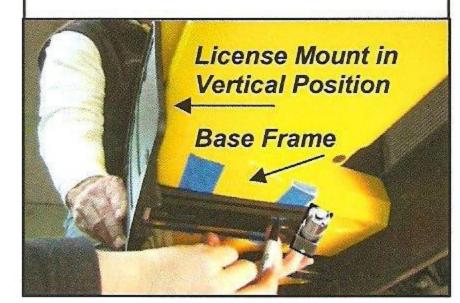
B. When the bottom of the bumper is deep enough, the base can be simply mounted using three screws
