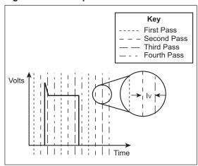
The CCP module is configured in Compare Special Event Trigger mode to accomplish this task. The phase shift is implemented by picking values of CCPRxL and CCPRxH that are not synchronous with the period of the sampling waveform. For instance, if the period of a waveform is 100  $\mu$ s, then sampling at a rate of once every 22  $\mu$ s will give the following set of sample times over 11 periods (all values in  $\mu$ s).
