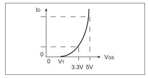
Low threshold devices commonly exist for MOSFETs with drain-to-source voltages rated below 30V. MOSFETs with drain-to-source voltages above 30V typically have higher gate thresholds (VT).
