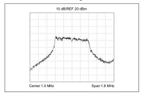
By spreading the energy over a wider range of frequencies, a drop of more than 20 dB is achieved.
