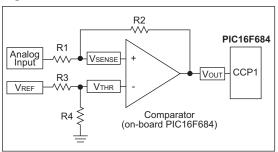
R3 and R4 set the threshold voltage for the comparator. When the analog input reaches the threshold voltage, Vout will toggle from low to high. R1 and R2 provide hysteresis to insure that small changes in the analog input won't cause jitter in the circuit. Figure 6-2 demonstrates the effect of hysteresis on the input. Look specifically at what Vsense does when the analog input reaches the threshold voltage.
