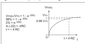
Now we need to estimate the capacitance. Capacitance is proportional to the area of a pixel. We can measure the area of a pixel and estimate the capacitance as shown. Obviously, a bigger display, such as a digital wall clock, will have bigger pixels and higher capacitance.
