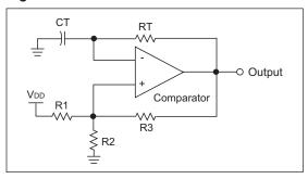
To design a multi-vibrator, first design the hysteresis feedback path using the procedure in Tip #3. Be careful to choose threshold voltages (VTH and VTL) that are evenly spaced within the common mode range of the comparator and centered on VDD/2. Then use VDD and VTL to calculate values for RT and CT that will result in the desired oscillation frequency Fosc. Equation 8-1 defines the relationship between RT, CT, VTH, VTL and Fosc.
