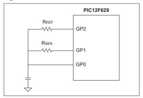
Other alternatives: voltage comparator in the PIC12F6XX to measure capacitor voltage on GP0.
