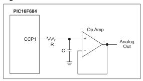
Pulse-width modulated signals can be used to create Digital-to-Analog (D/A) converters with only a few external components. Conversion of PWM waveforms to analog signals involves the use of an analog low-pass filter. In order to eliminate unwanted harmonics caused by a PWM signal to the greatest degree possible, the frequency of the PWM signal (FPWM) should be significantly higher than the bandwidth (FBW) of the desired analog signal. Equation 16-1 shows this relation.
