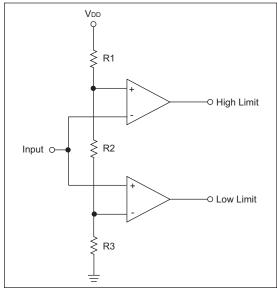
Resistors R1, R2 and R3 form a voltage divider which generates the high and low threshold voltages. The outputs HIGH LIMIT and LOW LIMIT are both active high, generating a logic one on the HIGH LIMIT output when the input voltage rises above the high threshold, and a logic one on the LOW LIMIT output when the input voltage falls below the low threshold.
