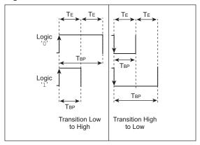
The figures show what a logic '0' or a logic '1' looks like for each modulation format. A transmission typically resembles an asynchronous serial transmission consisting of a Start bit, followed by 8 data bits, and a Stop bit.
