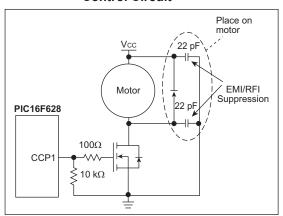
Figure 14-1 shows a unidirectional speed controller circuit for a brushed DC motor. Motor speed is proportional to the duty cycle of the PWM output on the CCP1 pin. The following steps show how to configure the PIC16F628 to generate a 20 kHz PWM with 50% duty cycle. The microcontroller is running on a 20 MHz crystal.
