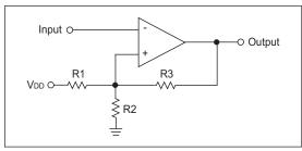
To calculate the resistor values required, first determine the high and low threshold values which will prevent chatter (V<sub>TH</sub> and V<sub>TL</sub>). Using V<sub>TH</sub> and V<sub>TL</sub>, the average threshold voltage can be calculated using the equation.
