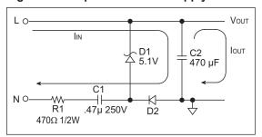
Figure 8-1 shows the basics for a capacitive power supply. The Zener diode is reverse-biased to create the desired voltage. The current drawn by the Zener is limited by R1 and the impedance of C1.
