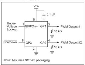
This design uses the PIC MCU comparator to implement an under-voltage lockout. The input on the GP0/C<sub>IN</sub>+ pin must be above the internal 0.6V reference for soft-start to begin, as shown in Figure 2-2.
