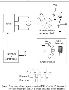
Quadrature sensing can easily be accomplished in software, but there is generally an upper limit to the RPM. By using a few gates, the sensing can be done partially in hardware and partially in software. The new PIC18FXX31 and dsPIC 16-bit Digital Signal Controller families include an encoder interface that allows MUCH higher RPM motors to be measured with an excellent degree of accuracy.
