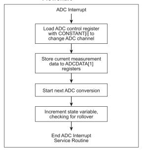
As shown in Figure 18-1, a constant array (CONSTANT[i]) can be created to store the values to be loaded into the ADC control register to change the ADC channel. Furthermore, a data array (ADCDATA[i]) can be used to store the results of the ADC conversion. Finally, the next conversion is started and the logic required to increment and bind the state variable is executed.
