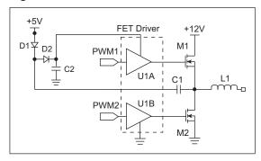
The +5V is used for powering the microcontroller. Using this arrangement, the FET driver would have approximately 12 + (5 - VDIODE) - VDIODE volts as a supply and is able to drive both the high and low side FETs.
