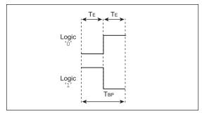
Figure 8-3: Pulse Position Modulation
