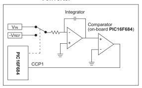
Dual-slope A/D conversion works by integrating the input signal (V<sub>IN</sub>) for a fixed time (T1). The input is then switched to a negative reference (-VREF) and integrated until the integrator output is zero (T2). V<sub>IN</sub> is a function of VREF and the ratio of T2 to T1.
