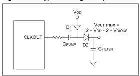
The PIC MCUs CLKOUT pin toggles at 1/4 of the oscillator frequency. When CLKOUT is low, D1 is forward biased and conducts current, thereby charging CPUMP. After CLKOUT is high, D2 is forward biased, moving the charge to CFILTER. The result is a voltage equal to twice the VDD minus two diode drops. This can be used with a PWM or any other I/O pin that toggles.
