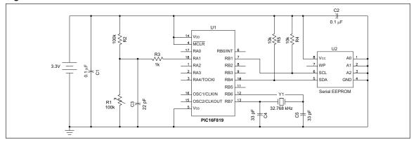
The system shown above is very simple and clearly has all the parts identified in the requirements. Unfortunately, it has a few problems in that the EEPROM, the sensor, and its bias circuit, are energized all the time. To get the minimum current draw for this design, it would be advantageous to shutdown these circuits when they are not required.
