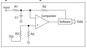
In operation, the feedback output from the software is a time sampled copy of the comparator output. In normal operation, the modulator output generates a PWM signal which is inversely proportional to the input voltage. As the input voltage increases, the PWM signal will drop in duty cycle to compensate. As the input decreases, the duty cycle rises.
