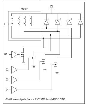
Figure 3-4: Bipolar Motor (4 Half-Bridges)
