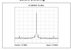
The PIC10F200 provides an Oscillator Calibration (OSCCAL) register that is used to calibrate the frequency of the oscillator. By varying the value of the OSCCAL setting, the frequency of the clock output can be varied. A pseudo-random sequence was used to vary the OSCCAL setting, allowing frequencies from approximately 600 kHz to 1.2 MHz. The resulting spectrum is shown in Figure 4-2.
