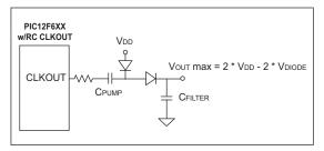
Voltages greater than VDD can be generated using a toggling I/O. PIC MCUs CLKOUT/OSC2 pin toggles at one quarter the frequency of OSC1 when in external RC oscillator mode. When OSC2 is low, the VDD diode is forward biased and conducts current, thereby charging CPUMP. After OSC2 is high, the other diode is forward biased, moving the charge to CFILTER. The result is a charge equal to twice the VDD minus two diode drops. This can be used with a PWM, a toggling I/O or other toggling pin.
