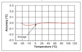
Figure 20-2 shows the average accuracy for the 100 sample lot of MCP9700 temperature sensors after compensation. The average error has been decreased over the full temperature range.
