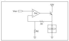
The voltage applied at the non-inverting terminal of the op amp is used to vary the voltage across the op amp. The non-inverting terminal voltage can be produced by a Digital-to-Analog Converter (DAC) or by the method shown in Tip #11.
