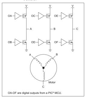
Figure 2-2: Back EMF Sensing (Sensorless Motor)
