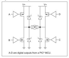
The H-Bridge derived its name from the common way the circuit is drawn. This is the only solid state way to operate a motor in both directions.
