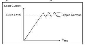
To design a PWM high current driver, first determine a switching speed (Fswx) that is appropriate for the system. Next, choose a MOSFET and D1 capable of handling the load current requirements. Then choose values for R2 and C1 using Equation 13-1.
