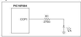
The CCP module, configured in PWM mode, is ideal for varying the intensity of an LED. Adjustments to the intensity of the LED are made by simply varying the duty cycle of the PWM signal driving the LED. This is accomplished by varying the CCPRxL register between 0 and 0xFF.
