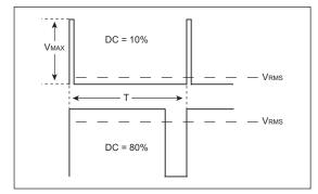
Equation 12-1 shows the relation between V<sub>RMS</sub> and V<sub>MAX</sub>.
