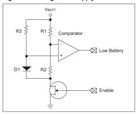
Comparator will trip when  $V_{BATT}$  = 3V: R1 = 33k, R2 = 10k and R3 = 470 $\Omega$ .
