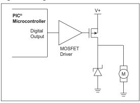
This drive can control a Brushed DC motor in one direction. This drive is often used in safety critical applications because a short circuit at the motor terminals cannot turn the motor on.
