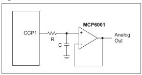
A PWM signal can be used to create a Digital-to-Analog Converter (DAC) with only a few external components. Conversion of PWM waveforms to analog signals involves the use of an analog low-pass filter. In order to eliminate unwanted harmonics caused by a PWM signal, the PWM frequency (FPWM) should be significantly higher than the bandwidth (FBW) of the desired analog signal. Equation 11-1 shows this relation.
