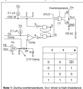
The block diagram for the MCP1630 high-speed PWM driver is shown in Figure 6-1. One of the features of the MCP1630 is the ability to
