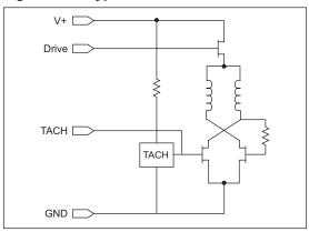
A 4-wire fan allows speed to be controlled using PWM via the Drive line. Since power to the tachometer sensor is not interrupted, it will continue to output the correct speed.
