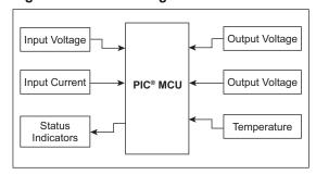
Using a PIC MCU as a controller allows for a greater level of intelligence in system monitoring. Rather than a single event causing a shutdown, a combination of events can cause a shutdown. A certain number of events in a certain time frame or possibly a certain sequence of events could be responsible for a shutdown.
