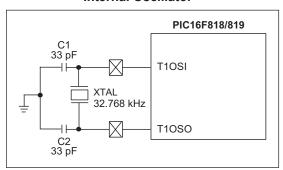
The calibration is based on the measured frequency of the internal RC oscillator. For example, if the frequency selected is 4 MHz, we know that the instruction time is 1  $\mu s$  (Fosc/4) and Timer1 has a period of 30.5  $\mu s$  (1/32.768 kHz). This means within one Timer1 period, the core can execute 30.5 instructions. If the Timer1 registers are preloaded with a known value, we can calculate the number of instructions that will be executed upon a Timer1 overflow.
