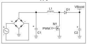
The AC voltage is rectified and boosted to voltages as high as 400 Vpc. The unique feature of the PFC circuit is that the inductor current is regulated to maintain a certain PF. A sine wave reference current is generated that is in phase with the line voltage. The magnitude of the sine wave is inversely proportional to the voltage at VBoost. Once the sine wave reference is established, the inductor current is regulated to follow it, as shown in Figure 7-2.
