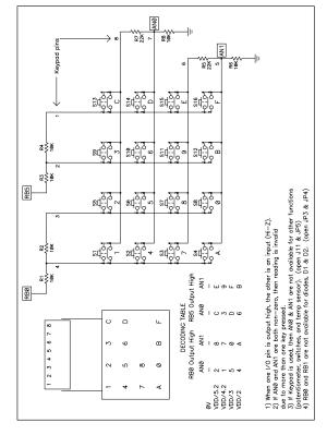
The two digital I/O pins that are used are RB0 and RB5, but any two digital I/O pins could work. The two analog pins used are AN0 and AN1.
