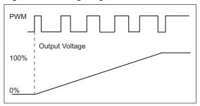
It is important to note that this type of soft-start controller can only be used for switching regulators that respond very quickly to changes on their shutdown pins (such as those that do cycle-by-cycle limiting). Some linear regulators have active-low shutdown inputs, however, these regulators do not respond fast enough to changes on their shutdown pins in order to perform soft-start.
