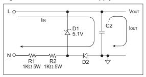
The resistive power supply works in a similar manner to the capacitive power supply by using a reversed-biased Zener diode to produce the desired voltage. However, R1 is much larger and is the only current limiting element.
