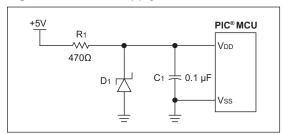
A simple, low-cost 3.3V regulator can be made out of a Zener diode and a resistor as shown in Figure 2-1. In many applications, this circuit can be a cost-effective alternative to using a LDO regulator. However, this regulator is more load sensitive than a LDO regulator. Additionally, it is less energy efficient, as power is always being dissipated in R1 and D1.
