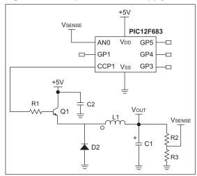
The design in Figure 16-1 utilizes an 8-pin PIC12F683 PIC MCU in a buck topology. The PIC12F683 has the basic building blocks needed to implement this type of power supply: an A/D converter and a CCP module.
