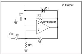
To design this multi-vibrator, first design the hysteresis feedback path using the procedure in Tip #3. Remember that the peak-to-peak amplitude of the ramp wave will be determined by the hysteresis limits. Also, be careful to choose threshold voltages (VTH and VTL) that are evenly spaced within the common mode range of the comparator.
