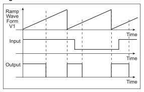
Figure 11-2: PWM Circuit
