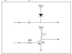
The two methods of producing a boost converter are shown above. The first circuit is simply a switched capacitor type circuit. The second circuit is a standard inductor boost circuit. These circuits work by raising VDD. This allows the voltage at VLCD to exceed VDD.
