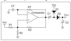
Note: The output voltage of a capacitive double is unregulated and will sag with increasing load current.
