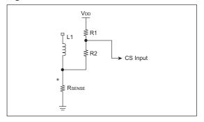
In this case, the Current Sense (CS) input of the MCP1630 is biased upward using the R1/R2 resistor divider. The equations for the new current limit are shown in Equation 6-2.
