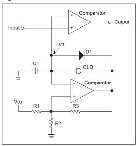
To design a PWM generator, start with the design of a ramp wave multi-vibrator using the design procedure from Tip #9. Choose high and low threshold voltages for the multi-vibrators hysteresis feedback that are slightly above and below the desired PWM control voltages.
