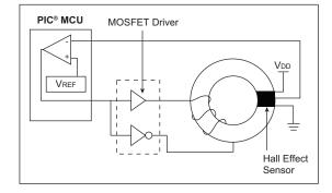
The Hall effect sensor output is proportional to the current being measured. When  $I_{IN} = 0$  amps, the output of the sensor will be  $V_{DD}/2$ . A current passing through the sensor in one direction will increase the output of the sensor, and a current in the other direction will decrease the output of the sensor.
