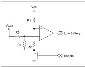
The comparator will trip when the battery voltage,  $V_{BATT} = 5.7V$ : R1 = 33k, R2 = 10k, R3 = 39k, R4 = 10k,  $V_{DD} = 5V$ .
