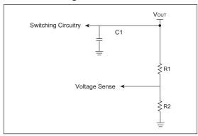
The output stage of many power supplies is similar to Figure 21-1. R1 and R2 are used to set the ratio of the voltage that is sensed and compared to the reference.
