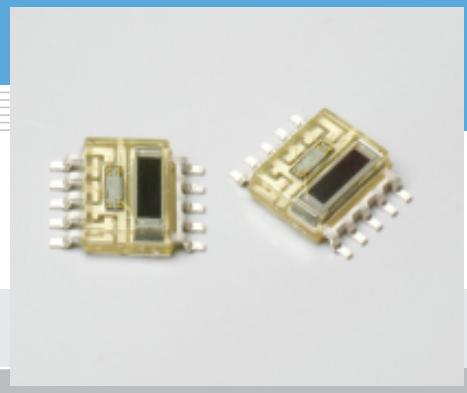
S10456 photo IC uses a dual-element Si PIN photodiode and compares the two signals to obtain a highly stable output. S10456 shows small variations in the propagation delay time even when laser power fluctuates, so that stable timing is output.
