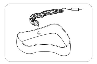
Figure 64. Typical wrist-type grounding strap.
