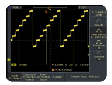
Figure 25. Example of an acquisition menu.
