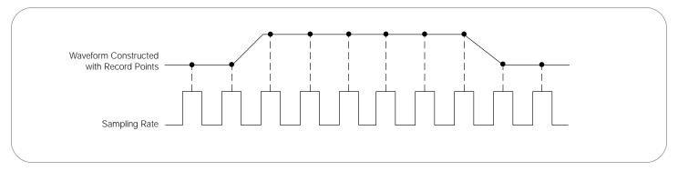
Figure 29. Real-time sampling method.
