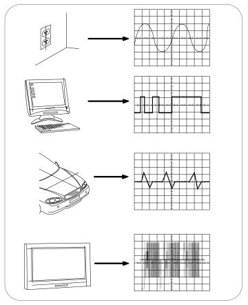
Figure 4. Sources of common waveforms.
