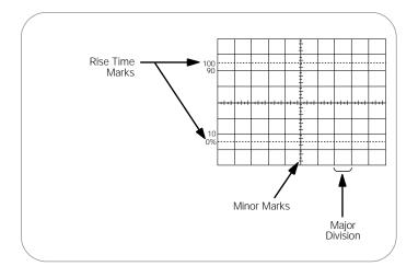
Figure 38. An oscilloscope graticule.
