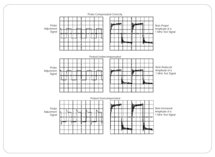
Figure 65. The effects of improper probe compensation.
