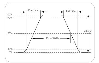
Figure 69. Rise time and pulse width measurement points.
