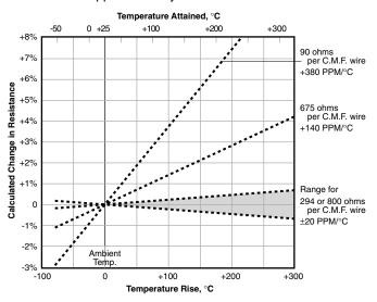
Fig. 15: Calculated change in resistance with nominal TC assumed constant.
