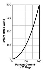
Fig. 1: Rapid increase of wattage with current or voltage.
