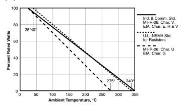
Fig. 3: Derating for ambient temperature.
