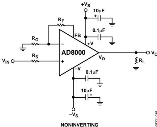
Figure 50. Noninverting Configuration
