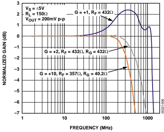
Figure 5. Small Signal Frequency Response vs. Various Gains
