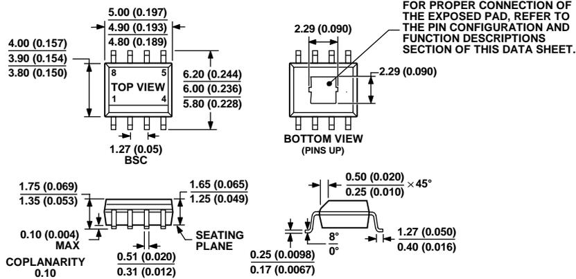
Figure 54. 8-Lead Standard Small Outline Package, with Exposed Pad [SOIC\_N\_EP] Narrow Body (RD-8-1)
