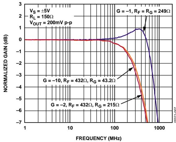
Figure 6. Small Signal Frequency Response vs. Various Gains
