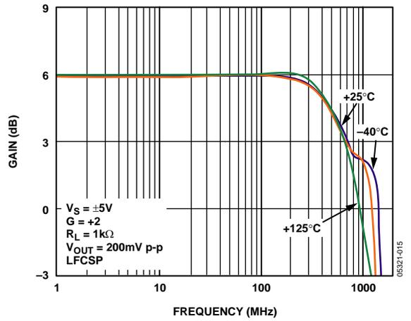
Figure 15. Small Signal Frequency Response vs. Temperature
