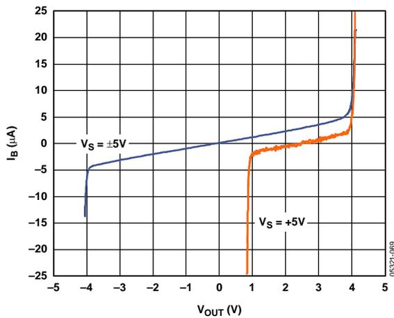
Figure 43. Input Bias Current vs. Output Voltage
