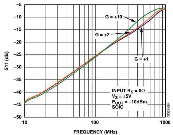
Figure 46. Input Voltage Standing Wave Ratio ( $S_{11}$ )
