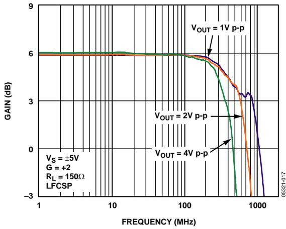
Figure 17. Large Signal Frequency Response vs. Various Outputs
