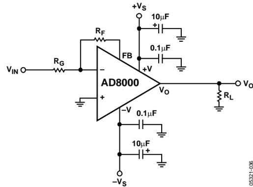
Figure 51. Inverting Configuration
