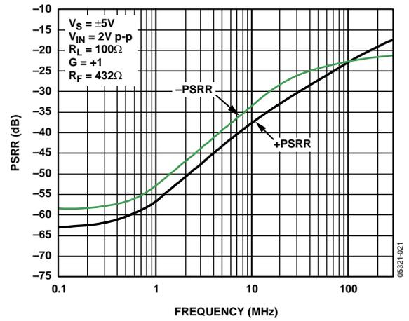
Figure 32. Power Supply Rejection Ratio (PSRR) vs. Frequency
