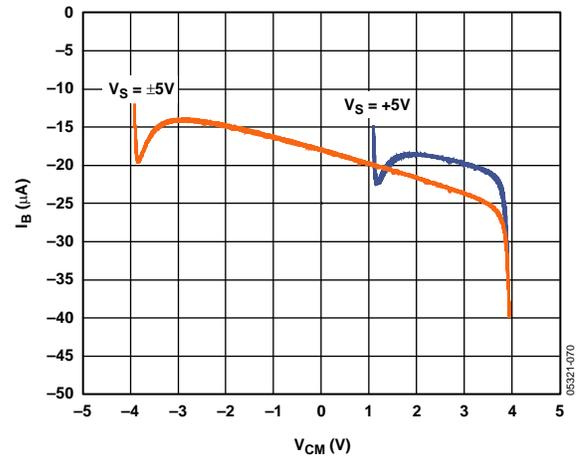
Figure 44. Input Bias Current vs. Common-Mode Voltage
