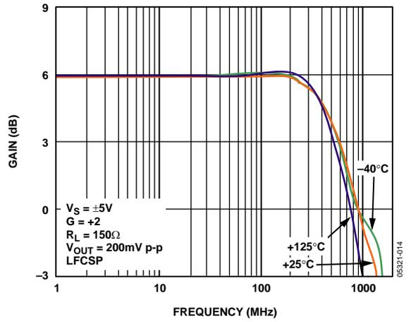
Figure 14. Small Signal Frequency Response vs. Temperature
