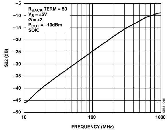
Figure 45. Output Voltage Standing Wave Ratio ( $S_{22}$ )
