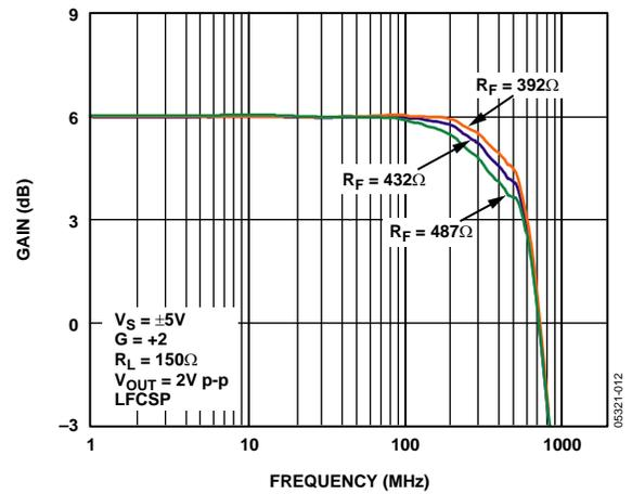
Figure 9. Large Signal Frequency Response vs.  $R_F$
