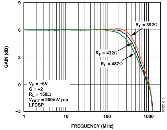
Figure 8. Small Signal Frequency Response vs.  $R_F$
