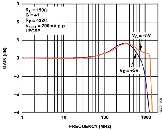
Figure 12. Small Signal Frequency Response vs. Supply Voltage
