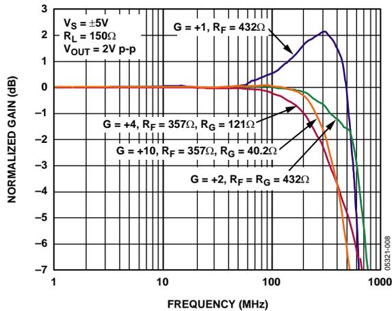
Figure 7. Large Signal Frequency Response vs. Various Gains
