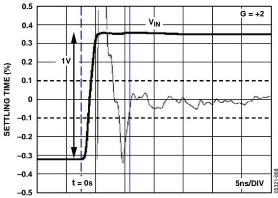
Figure 36. Settling Time
