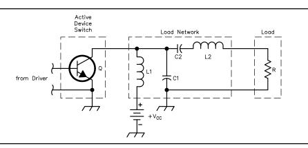
Fig 2—Schematic of a low-order Class-E amplifier.
