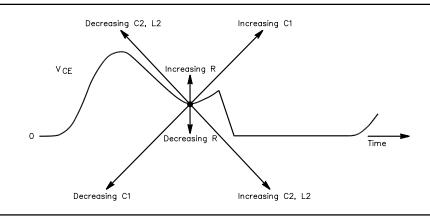
Fig 5—Effects of adjusting load-network components.
