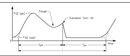
Fig 4—Typical mistuned V waveform, showing transistor turn-on, turn-off and waveform "trough."
