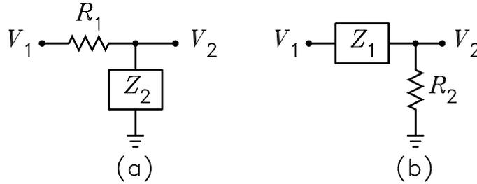
Figure 5: Voltage divider networks containing only one capacitor.
