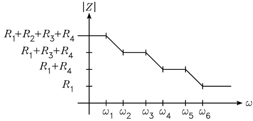
Figure 3: Bode magnitude plot for the impedance  $Z$ .
