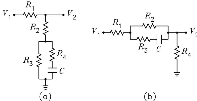
Figure 6: Example circuits for the voltage-divider theorem.
