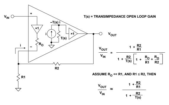
Figure 2: Current Feedback (CFB) Op Amp Topology
