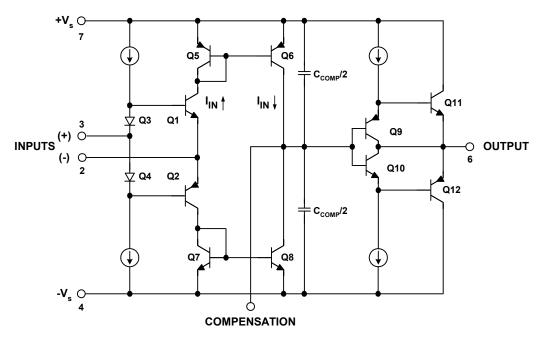
Figure 3: AD846 Current Feedback Op Amp (1988)
