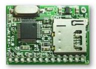
$\mu ALFAT^{TM}$  is an OEM board of  $\mu ALFAT^{TM}$  chip with TransFlash (micro SD) card connector. It has very small dimensions which makes it ideal for small data logger. This OEM board is one of the smallest OEMs with high performance file system abilities , about 1" by 1.4"!
