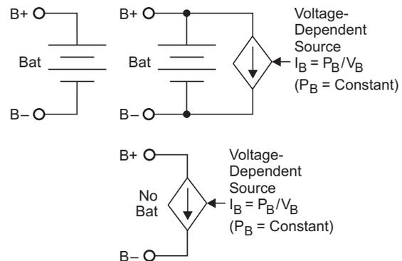
Fig. 28. Expected loads for an embedded battery charger.
