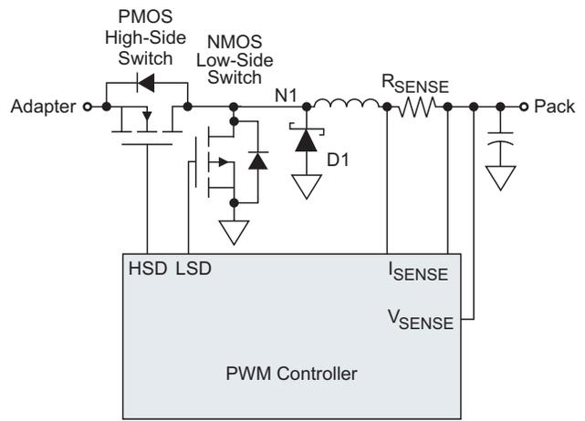
Fig. 7. Synchronous topology with a PMOS high-side switch.
