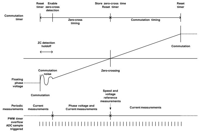
The sensorless commutation control is implemented using several interrupts. Interrupts are enabled and disabled during different stages of the commutation cycle. Table 3 shows the responsibility of each interrupt. The state diagram in **Figure** 9 shows how the interrupts cooperate to perform sensorless commutation.
