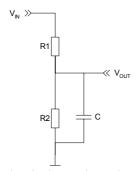
The component values in this circuit depend on the desired DC gain and low pass filter corner frequency. The following observations should assist the choice of components:
