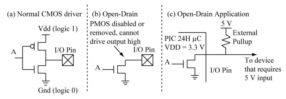
$_{\text{ODC}}xy = 1$  enables open drain,  $_{\text{ODC}}xy = 0$  disables open drain
