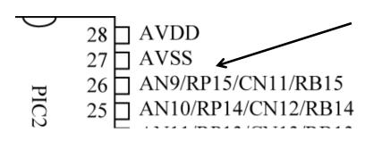
RB15 shared with AN9, which is an analog input to the on-chip Analog-to-Digital Converter (ADC). Must disable analog functionality!
