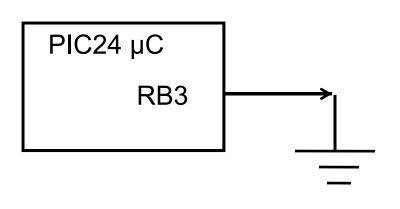
Configure RB3 as an open-drain output, then write a '1' to it.
