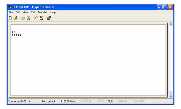
3. Select Transfer>Send File... on the Menu Bar and at the Send File prompt, select the firmware upgrade file (.ROM file), select the Xmodem protocol and press the "Send" button
