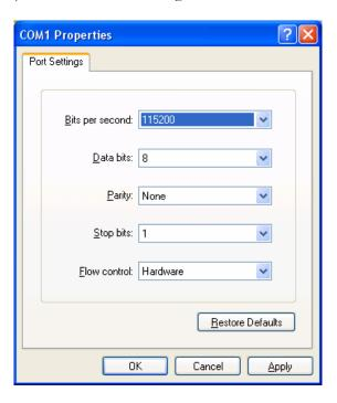
5. On the menu bar, select "File>Properties" and click on the "Settings" tab and select the "ASCII Setup..." button. Then choose the settings as shown:
