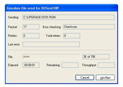
5. After the file transfer completes and there are no errors, the new firmware will be executed. Enter two <CR>'s (press the Enter key twice) to complete the CD17B10's autobaud detection.
