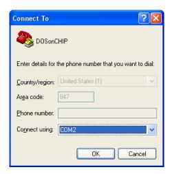
4. At the next prompt, choose the serial port speed (see the CD17Bxx User Guide for allowable serial speeds), and choose the settings as shown:
