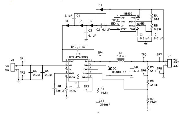
Figure 6. Charge Pump Circuit for TPS54240EVM-605
