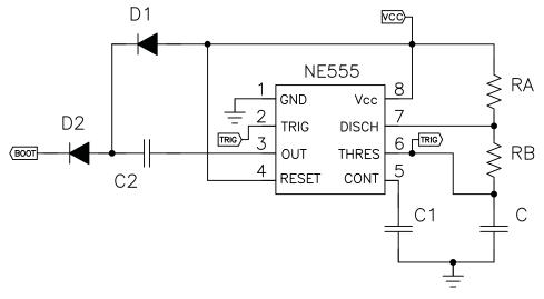
Figure 4. NE555 Charge Pump Circuit
