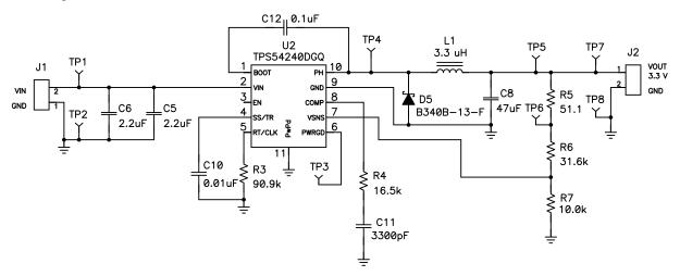
Figure 1. TPS54240 Test Configuration
