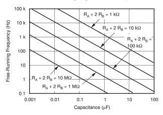
Figure 5. Free-Running Frequency of the 555 Timer
