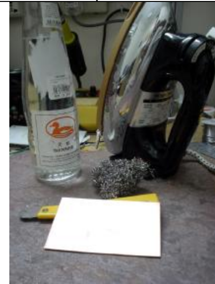
Items required: Blank PCB, iron, scouring pad (stainless steel), paint thinner
