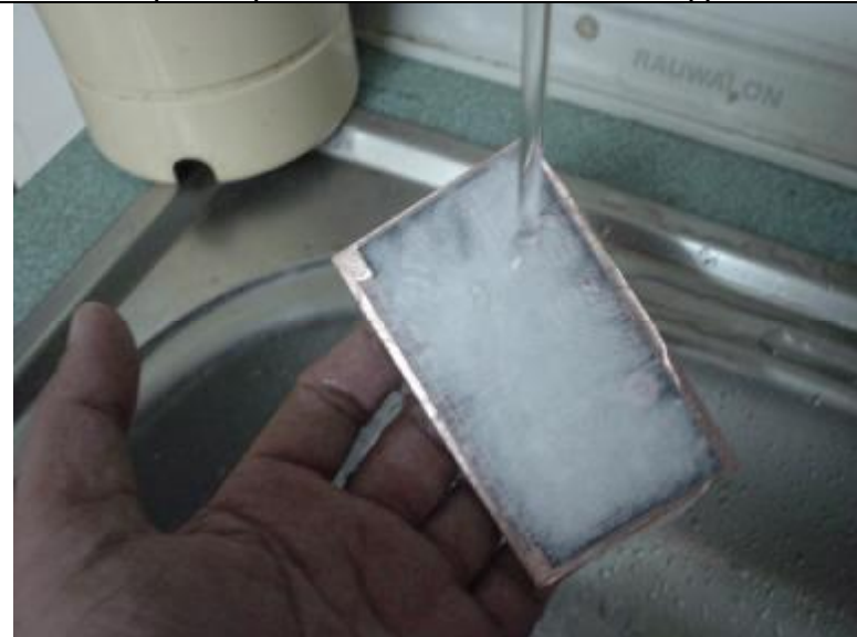
After initial removal then gently remove remaining paper
