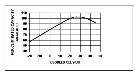
Charging nickel cadmium cells below the recommended temperature can cause oxygen pressure build up and activation of the resealable safety vent. Multiple vent activations will reduce cell capacity.
