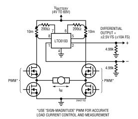
Figure 3. LTC6103 Provides Bidirectional H-Bridge Monitoring with ADC-Friendly Differential Output
