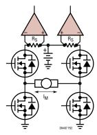
Figure 2. PWM-Compatible H-Bridge Load Sensing
