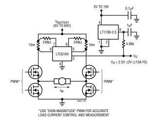
Figure 4. LTC6104 Provides Bidirectional H-Bridge Monitoring with Single-Ended Output
