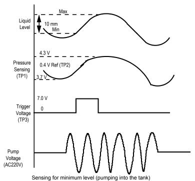
The sensing probe is tied to the positive pressure port of the sensor. The pump is turned on to fill the tank when the minimum level is reached.
