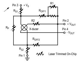
Figure 1. Pressure Sensor MPXM2000 Series
