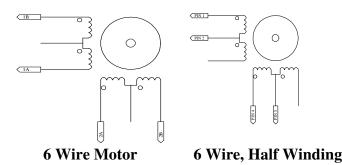
Unipolar drivers, as described previously, do not have the capability to reverse the current flow. In order to make the motor operate as desired, the 2 center taps of a 6 lead motor (see diagram "6 Wire Motor") are connected to the supply voltage. By simply switching either of the end taps to GND, the driver can generate a current in either direction within the coil. As a result, only ½ of the coil will be operated at a given time.
