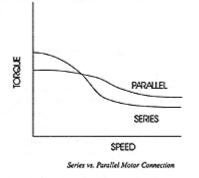
In case of a six lead motor, the performance at higher speeds can be improved by using the below half winding configuration. This comes at the price of reduced torque at lower and mid range speeds. However, due to the reduced inductance, performance at higher speeds is improved.
