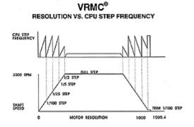
Microstepping is typically used in applications that require accurate positioning and a fine resolution over a wide range of speeds.
