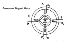
Unlike the other stepping motors, the PM motor rotor has no teeth and is designed to be magnetized at a right angle to it's axis. The above illustration shows a simple, 90 degree PM motor with four phases (A-D). Applying current to each phase in sequence will cause the rotor to rotate by adjusting to the changing magnetic fields. Although it operates at fairly low speed the PM motor has a relatively high torque characteristic.
