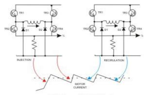
Bipolar Chopper Drive Switch Circuit
