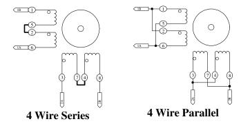
A series connection provides a high inductance and therefore greater performance at low speeds. A parallel connection will lower the inductance but increase the torque at faster speeds. The following is a typical speed/torque curve for an AMS driver and motor connected in series and parallel:
