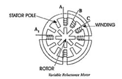
The variable reluctance motor in the above illustration has three "stator pole sets" (A, B, C,), set 15 degrees apart. Current applied to pole A through the motor winding causes a magnetic attraction that aligns the rotor (tooth) to pole A. Energizing stator pole B causes the rotor to rotate 15 degrees in alignment with pole B. This process will continue with pole C and back to A in a clockwise direction. Reversing the procedure (C to A) would result in a counterclockwise rotation.
