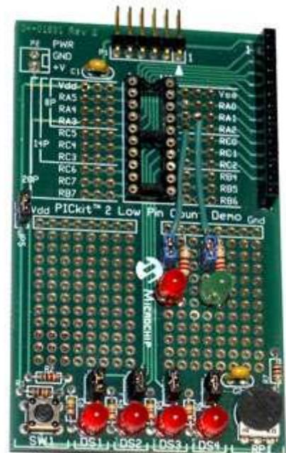
capacitor (C1) across the power pins. Power (5 V) is supplied from the PICKit 2.
