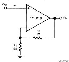
\*R not needed due to temperature independent  $I_{\text{IN}}$
