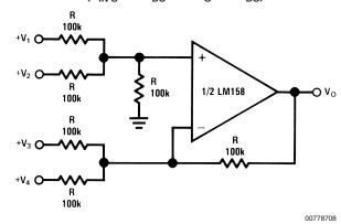
Where:  $V_0 = V_1 + V_2 - V_3 - V_4$  $(V_1 + V_2) \ge (V_3 + V_4)$  to keep  $V_O \ge 0$   $V_{DC}$
