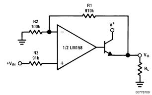
$V_O = 0 V_{DC}$  for  $V_{IN} = 0 V_{DC}$  $A_{V} = 10$
