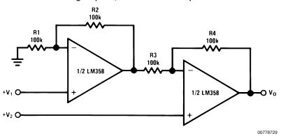
For  $\frac{R1}{R2} = \frac{R4}{R3}$  (CMRR depends on this resistor ratio match)  $V_O = 1 + \frac{R4}{R3} (V_2 - V_1)$ As Shown:  $V_O = 2 (V_2 - V_1)$
